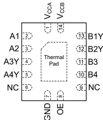
**Figure 4-2. Pin Diagram (VQFN-14 Package)**
