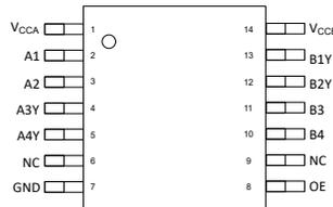
**Figure 4-1. Pin Diagram (TSSOP-14) Package**
