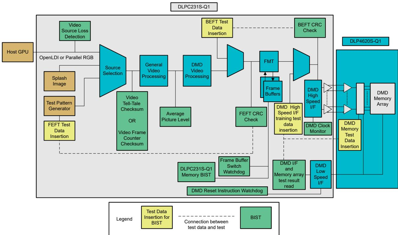
**Figure 6-1. DLP4620S-Q1 Video Path With Diagnostics**
