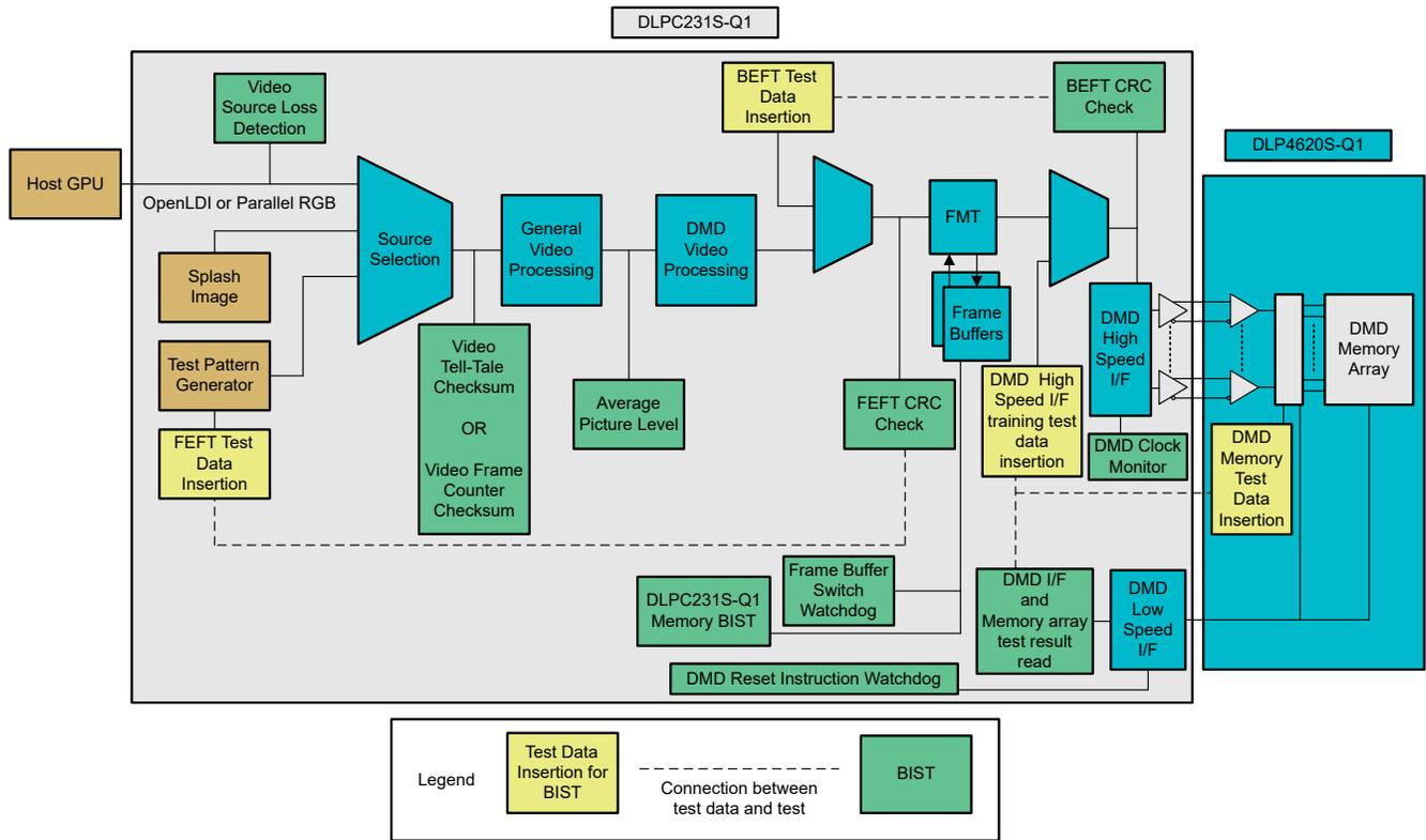
Figure 4-2. DLP4620S-Q1 Video Path With Diagnostics
