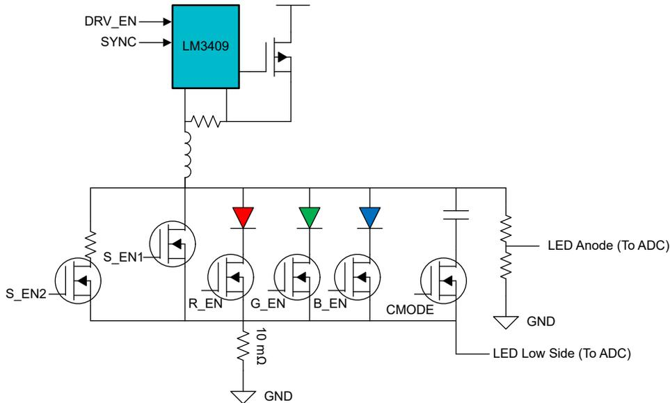
**Figure 6-7. LED Driver Architecture**
