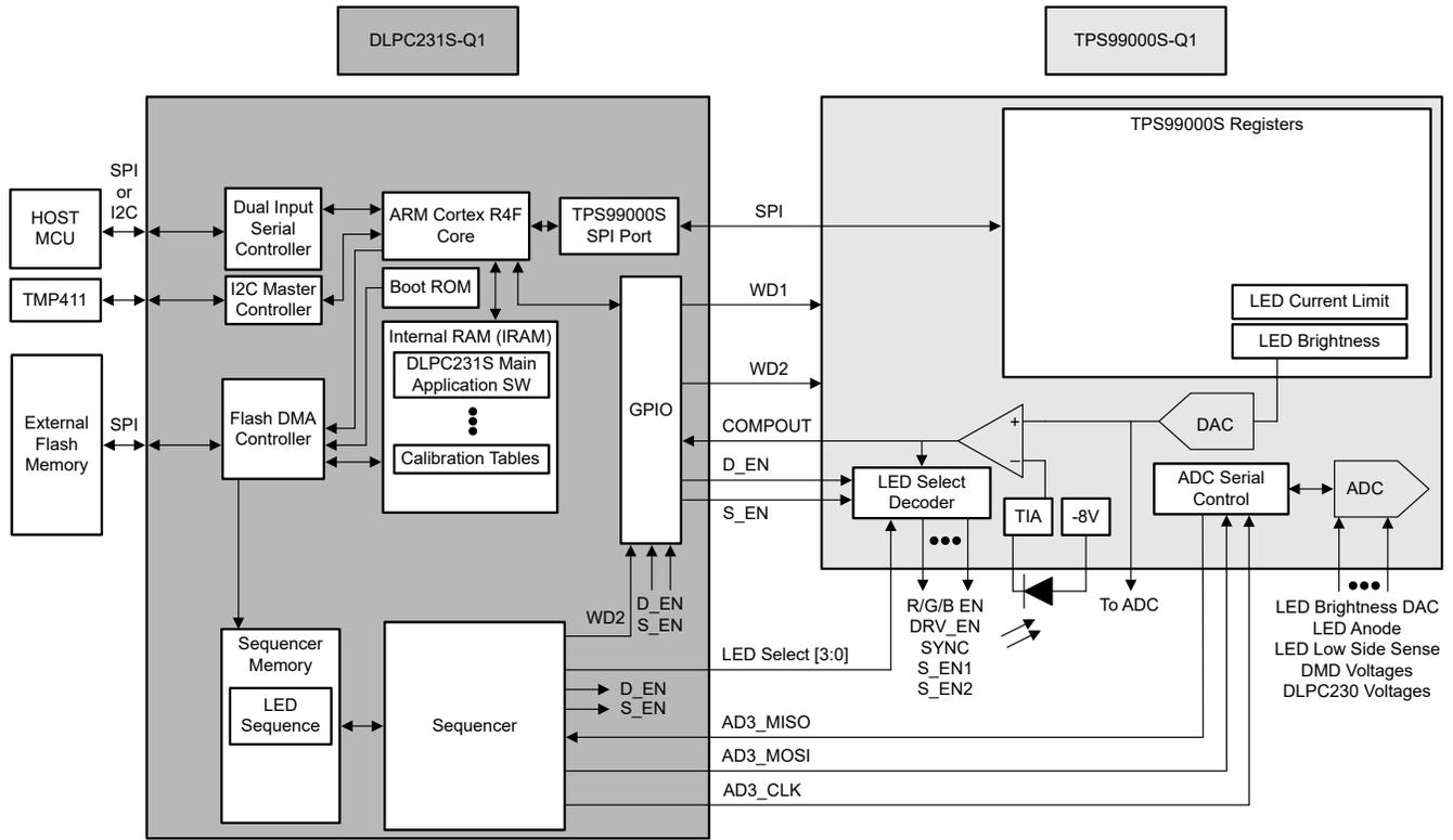
**Figure 6-6. Illumination Control Architecture**
