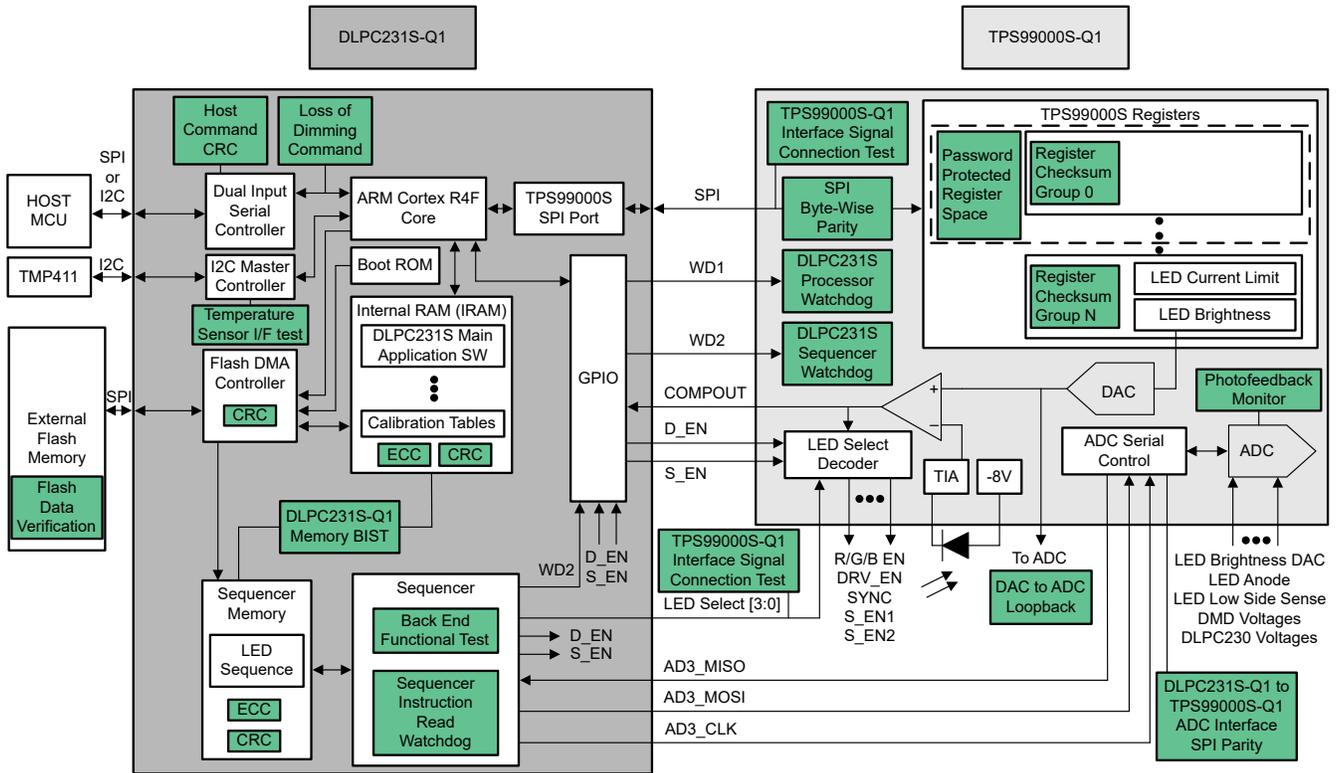
Figure 6-9. Illumination Control Architecture With Diagnostics
