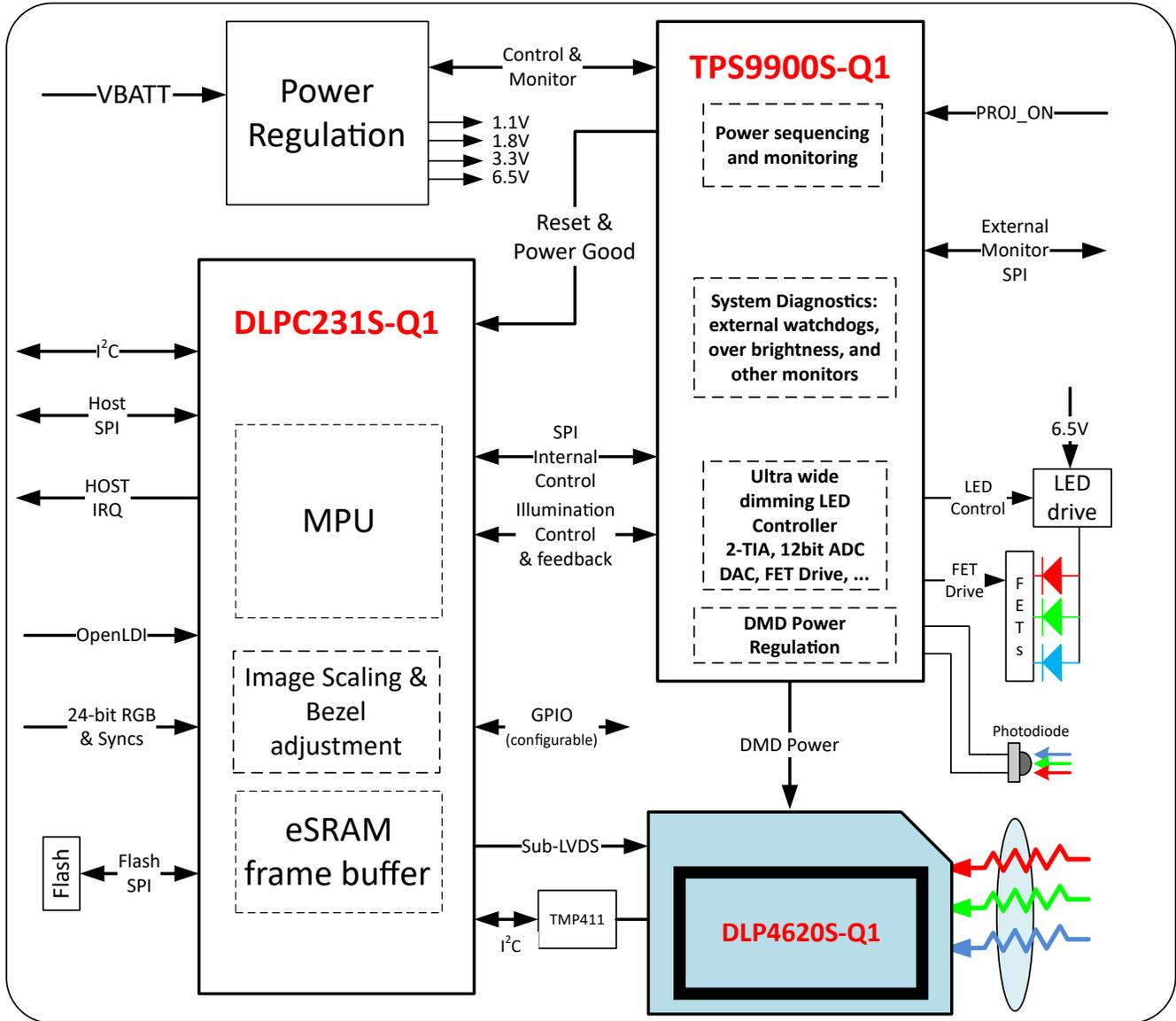
Figure 4-1. DLP4620S-Q1 Chipset Block Diagram
