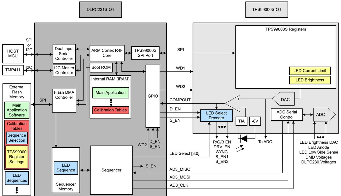
Figure 6-8. Software and Settings Origin and Destination
