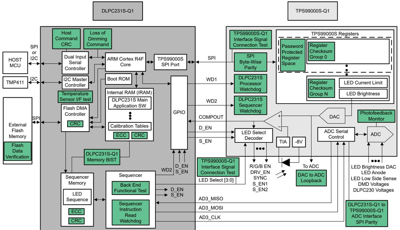
Figure 4-3. Illumination Control Architecture With Diagnostics
