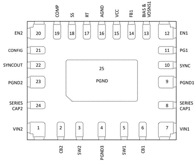
**Figure 4-2. Single Primary Pin Diagram**
