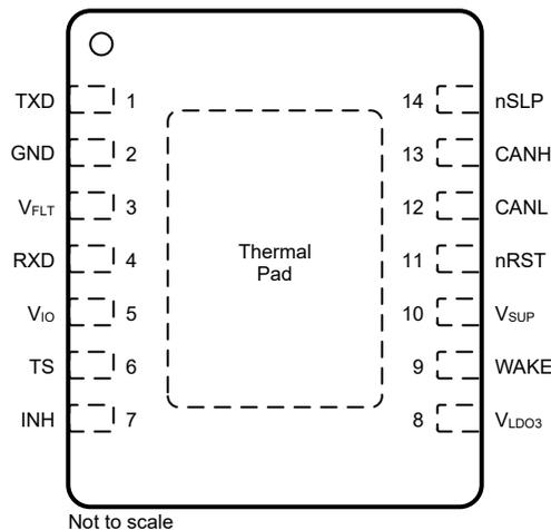
**Figure 4-1. Pin Diagram (TCAN11623-Q1 DMT) Package**
