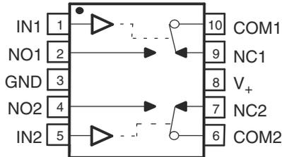
**Figure 1-1. Functional Block Diagram**
