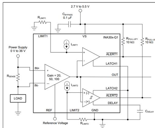
Figure 1-1. Functional Block Diagram
