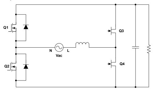
Figure 3-1. Basic Totem Pole PFC Circuit Structure
