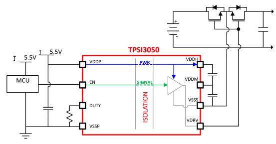
Figure 2-1. TPSI3052 Simplified Schematic
