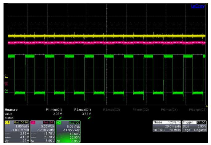
A. CH1 (Yellow): 3.3V Input, CH2 (Red): Vdrv Pin, CH4 (Green): PFC low-side Vgs
