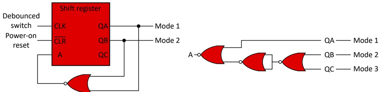
**Figure 3. Single Input for Mode Control and Device Enable**
