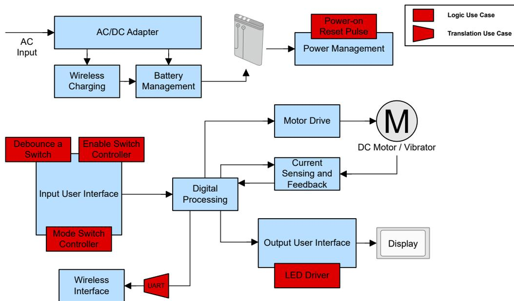
Figure 1. Simplified Block Diagram for Personal Care Electronics
