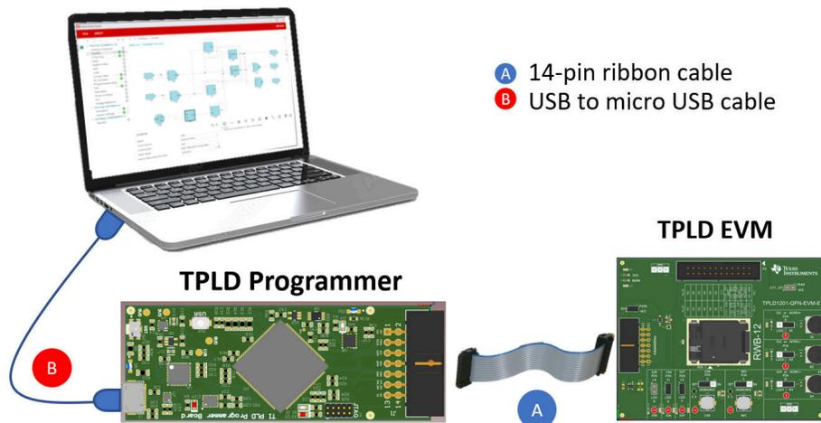
**Figure 2-3. TPLD-PROGRAM Hardware Connections**
