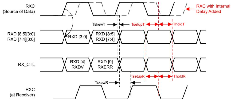
**Figure 3. RGMII Version 1.3 and 2.0 Receiver Timing Diagram**
