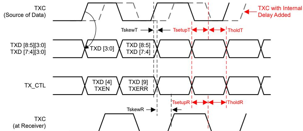
**Figure 2. RGMII Version 1.3 and 2.0 Transmitter Timing Diagram**
