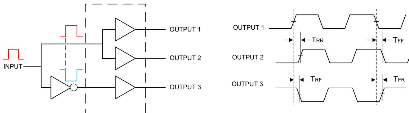
**Figure 4. Output Skew ( $T_{RR}/T_{FF}$ ) and Inverting Skew ( $T_{RF}/T_{FR}$ ) Measurements**
