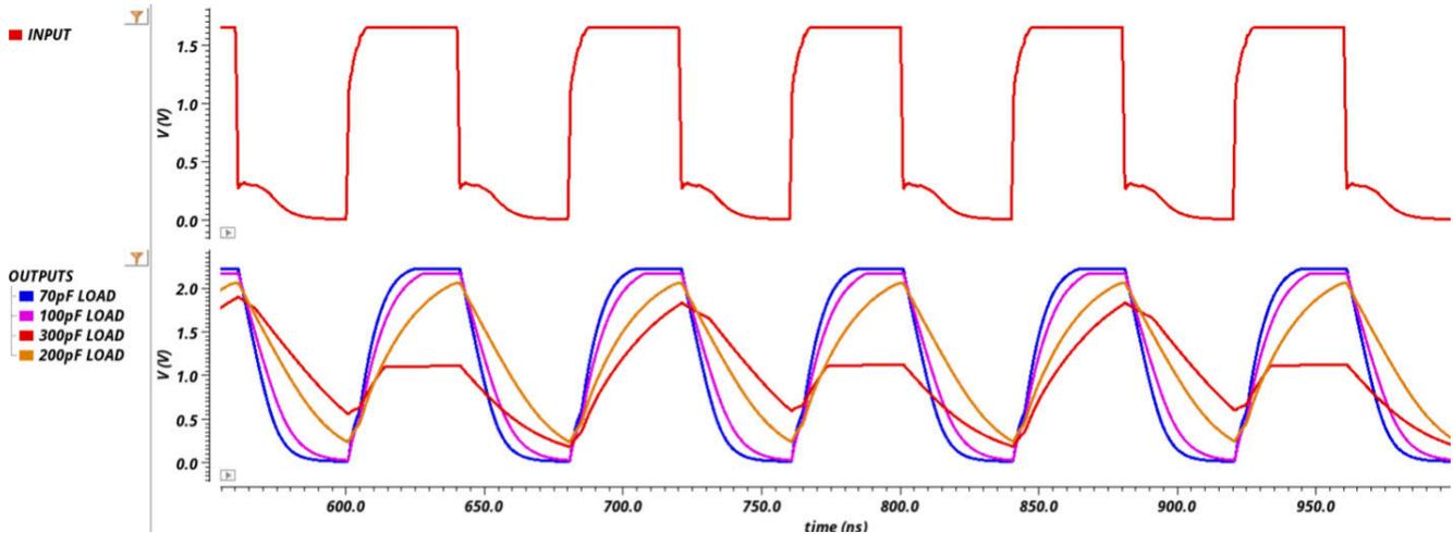
Figure 5-1. Example Voltage Translation showing Lumped Capacitance with a One-Shot Device
