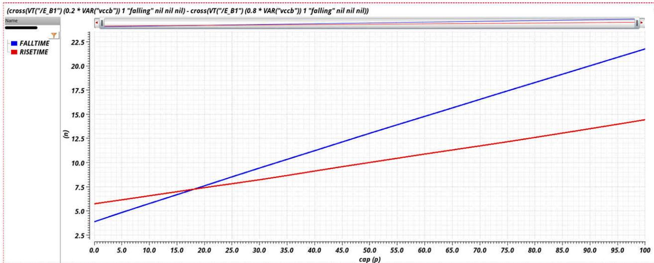
Figure 4-1. Example of Rise and Fall Times Increasing with Lumped Capacitance
