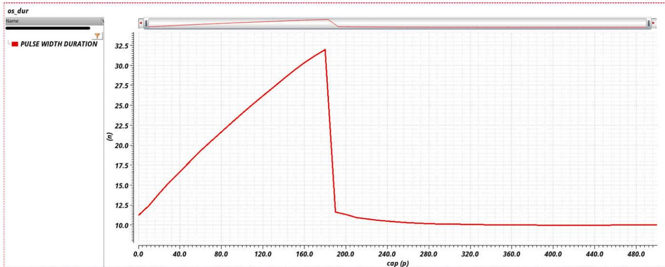
Figure 2-1. Example of the one-shot timing out before reaching the designed duration.
