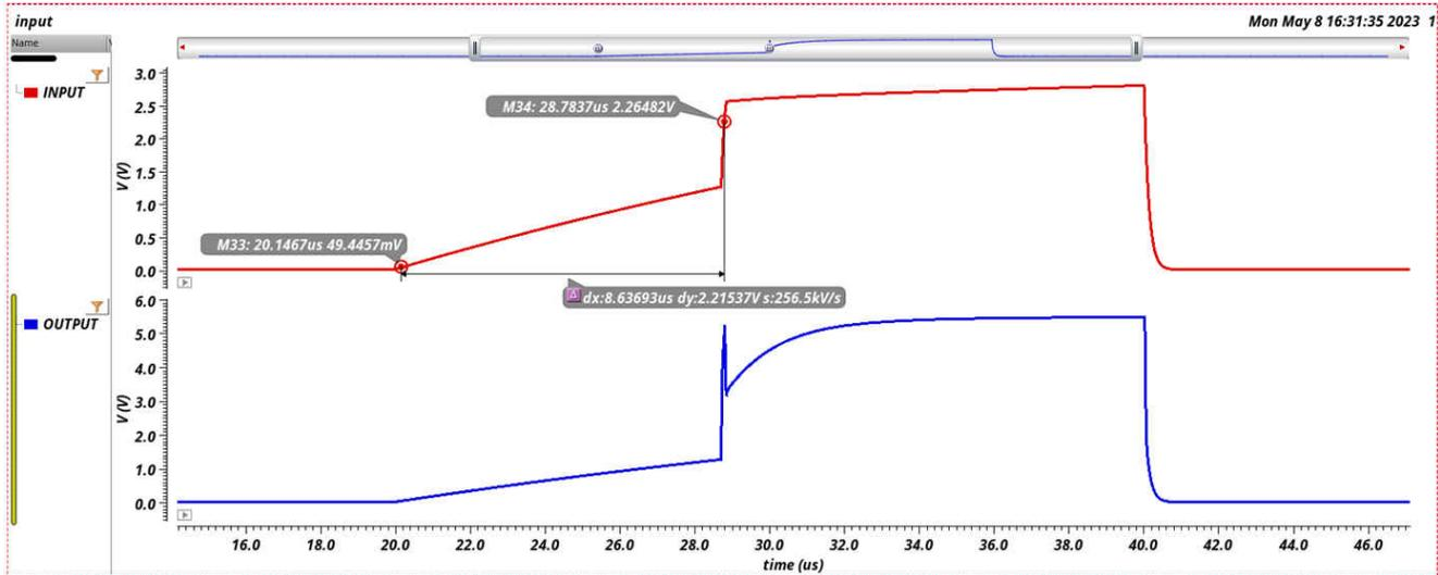
Figure 3-1. Example of Slow Rise and Fall Times, 2.4  $\mu\text{s/V}$
