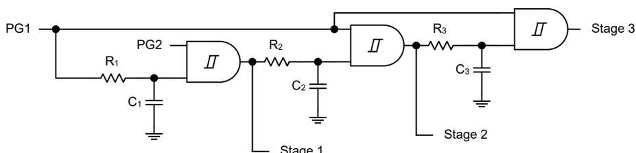
**Figure 2. Example Logic Circuit for Sequencing Components**
