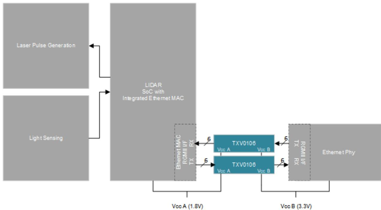
**Figure 2. RGMII for LIDAR SoC Application**
