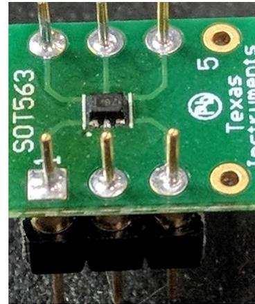
Figure 4. Soldered SN74AXC1T45DRL With Header Pins
