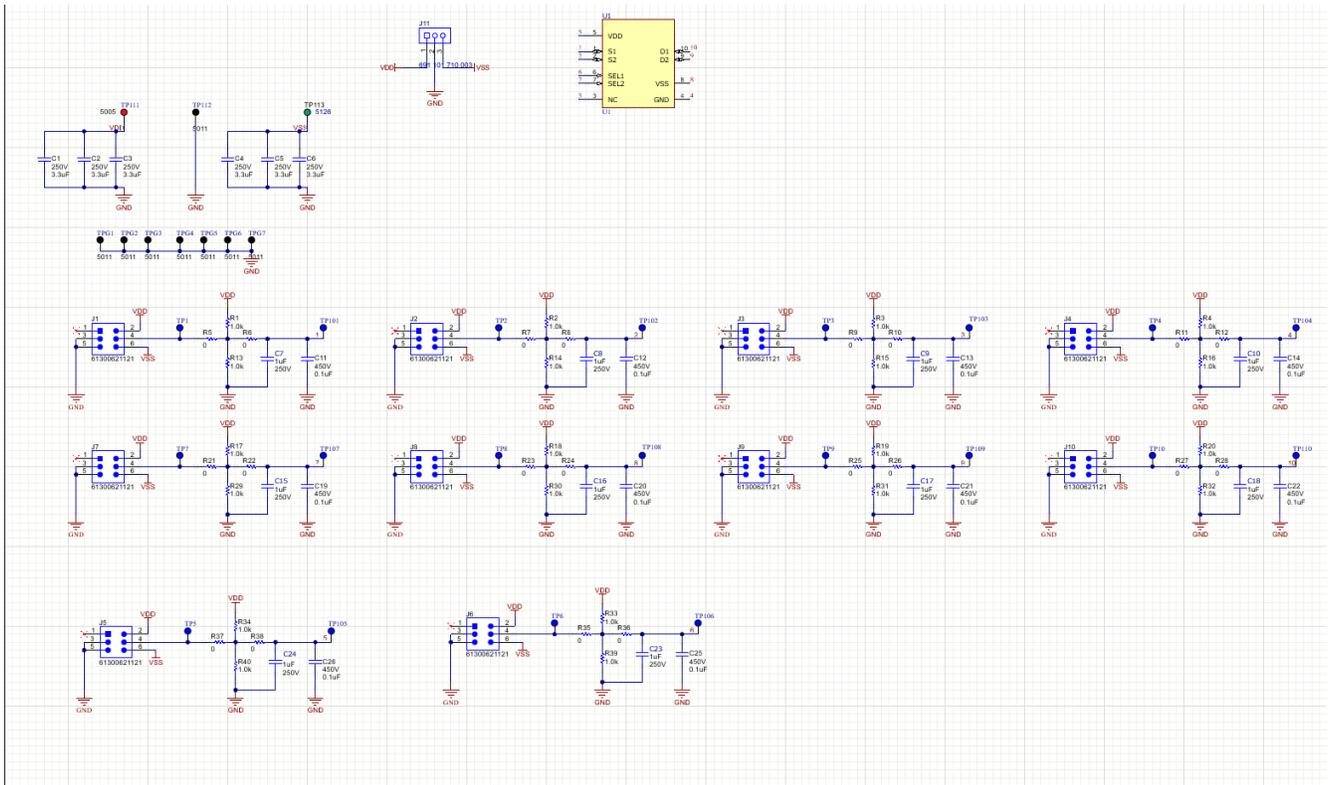
Figure 3-1. Main Schematic – TMUX10DGS All Components Shown
