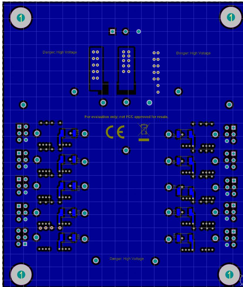
Figure 3-4. TMUX10DGSEVM Bottom Layer Layout
