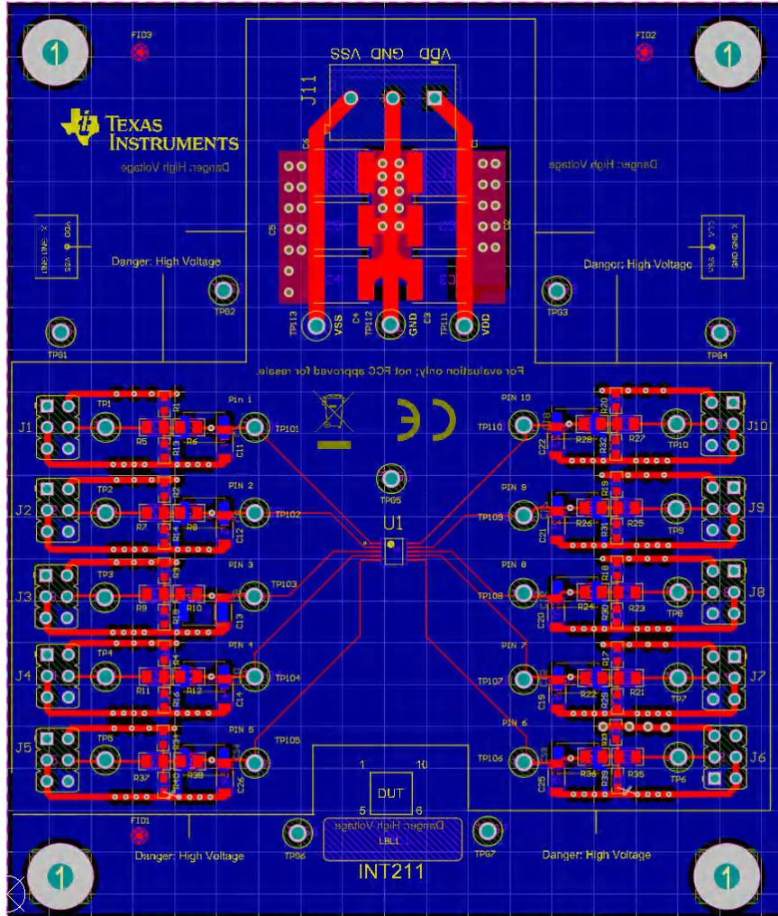
Figure 3-3. TMUX10DGSEVM Top Layer Layout
