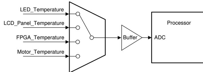
**Figure 1-1. Expansion of 1 MCU ADC Input to 4 Sensor Outputs for Monitoring Using a Multiplexer**
