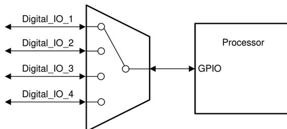
**Figure 2-1. Expansion of 1 MCU GPIO to Four Digital I/Os Using A Multiplexer**
