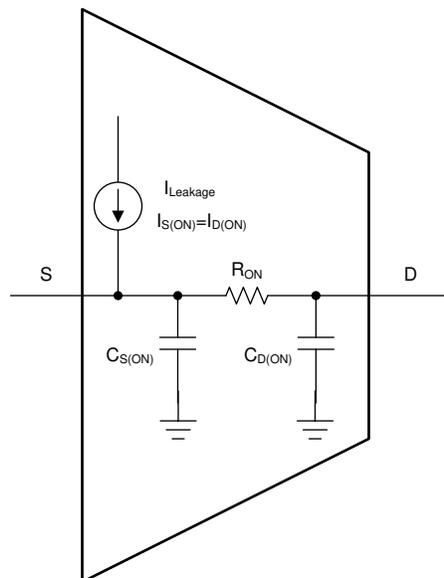
**Figure 1-2. Simplified Circuit Model of FET Switch When Signal Switch is Selected**
