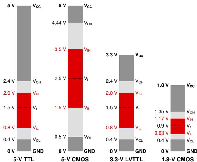
Figure 1. Logic Thresholds
