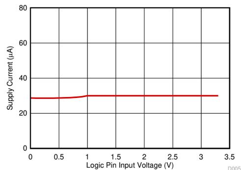
**Figure 7. Fixed Threshold  $I_{CC}$  vs Logic Input Voltage**
