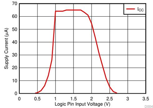
**Figure 6. 1.8-V Compatible  $I_{CC}$  vs Logic Input Voltage**
