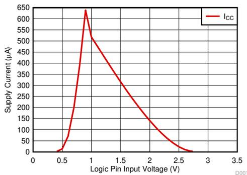
**Figure 5. 70% or 30% Threshold  $I_{CC}$  vs. Logic Input Voltage**
