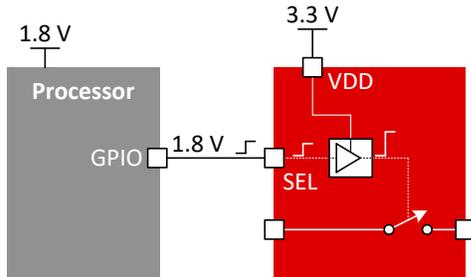
**Figure 4. MUX or Switch With Integrated 1.8-V Logic**
