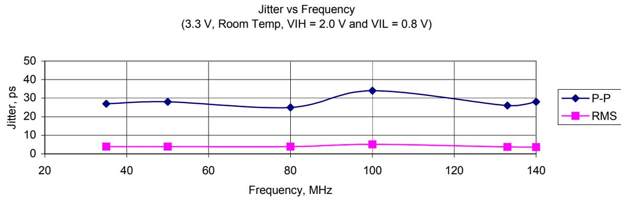
**Figure 3. Peak-to-Peak and RMS Jitter of CDCV304 Driver Output (Point 2)**
