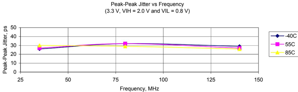
**Figure 4. Peak-to-Peak Jitter of CDCV304 Driver Output (Point 2 Over Industrial Temperature Range)**
