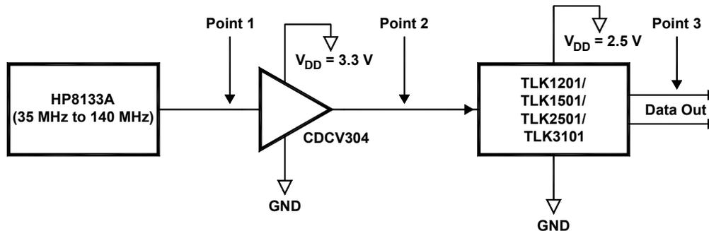
**Figure 5. Test Equipment Setup**
