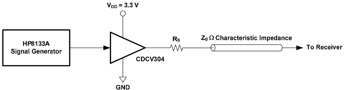
**Figure 6. Series Termination for CDCV304 Clock Driver**
