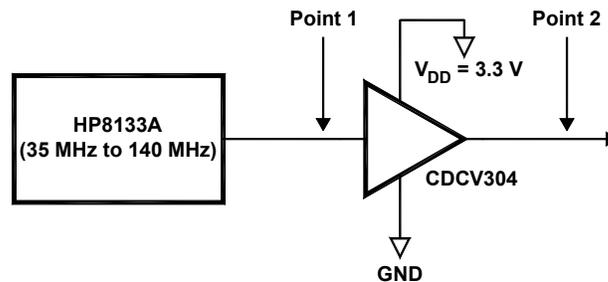
**Figure 1. Indicates Various Jitter Measurement Points**
