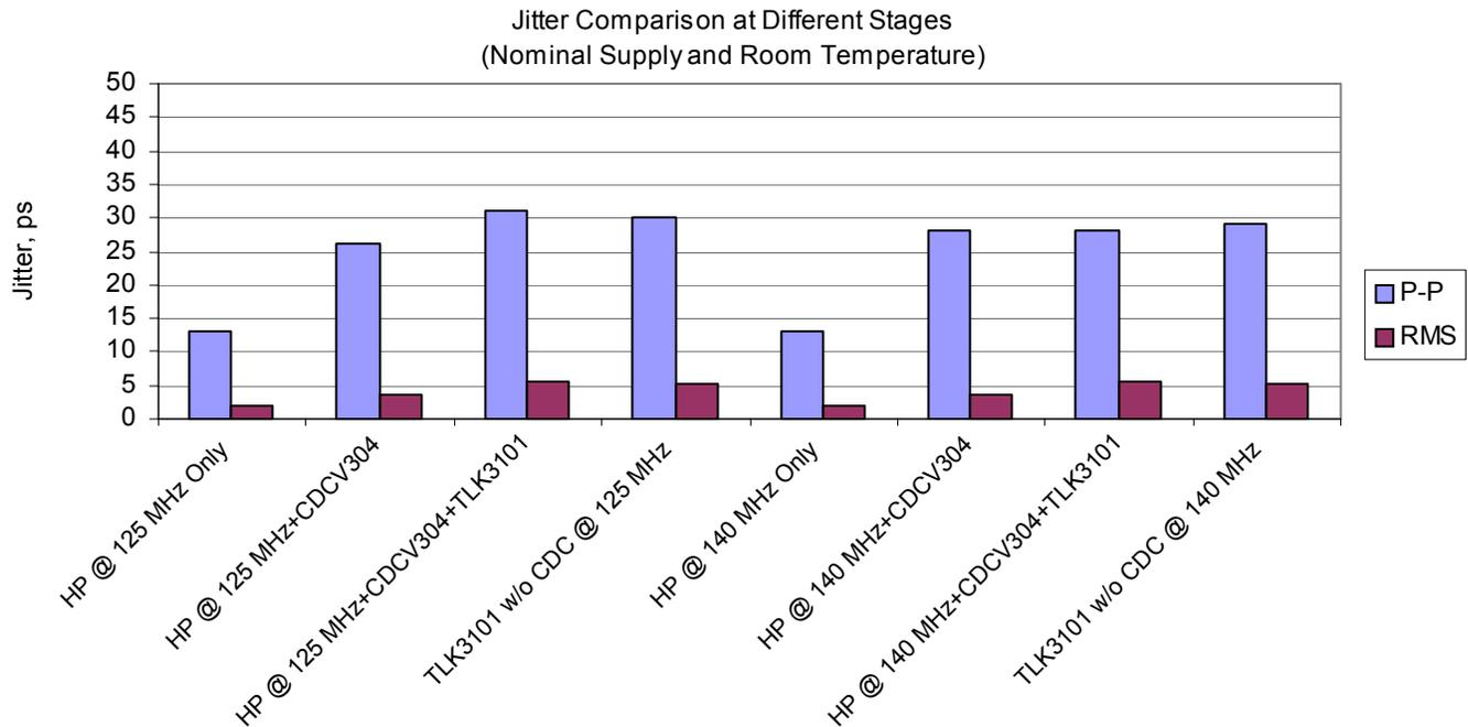
Figure 10. Jitter Values at Different Points Shown in Figure 5 With TLK3101
