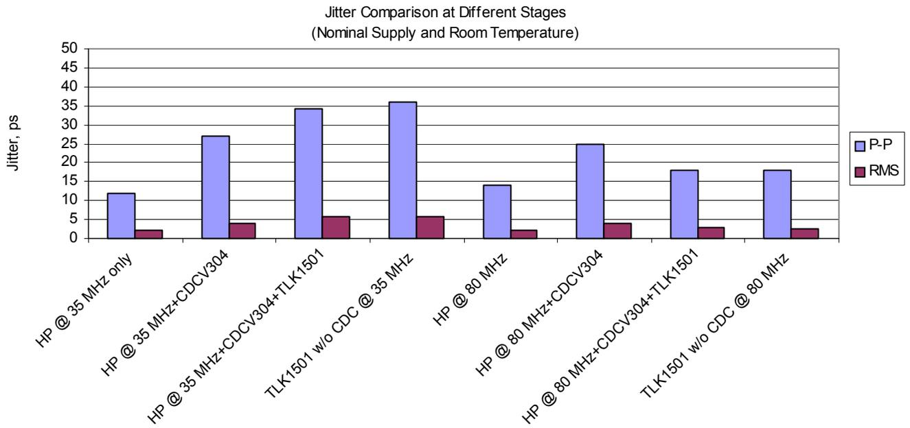
Figure 8. Jitter Values at Different Points Shown in Figure 5 With TLK1501
