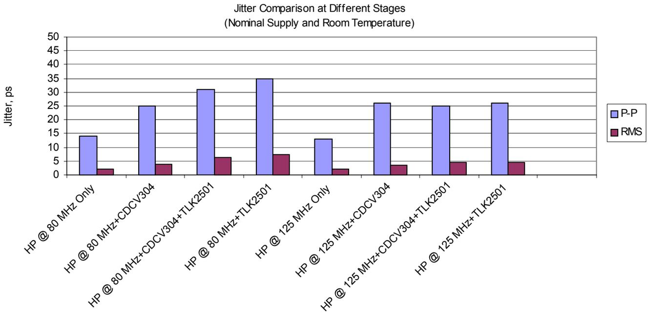
**Figure 9. Jitter Values at Different Points Shown in Figure 5 With TLK2501**
