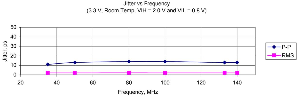
**Figure 2. Peak-to-Peak and RMS Jitter of HP Signal Generator (Point 1)**
