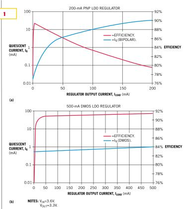
Even a so-called micropower regulator with a pnp pass element and a featured quiescent current of 20  $\mu$ A can draw 30 mA, or 13% of its rated supply current, at its maximum rated load of 200 mA (a). A DMOS LDO regulator, the REG103, features a quiescent-current draw of 1 mA at the full-rated, 500-mA load (b).
