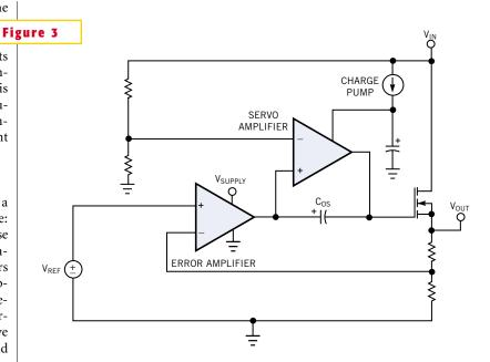
A new topology uses a fast voltage-control amplifier to control the gate and a slow servo amplifier to maintain the proper offsetting voltage across a dc level-shift, or offsetting, capacitor, C<sub>oc</sub>.
