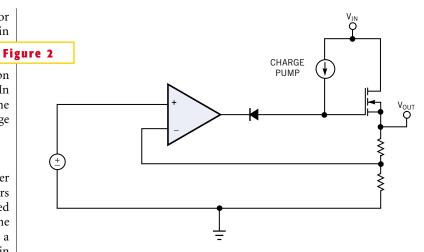
A previous approach to driving an n-type-DMOS pass element uses a charge pump to directly drive the gate, which leads to high noise and limited positive slew rate.
