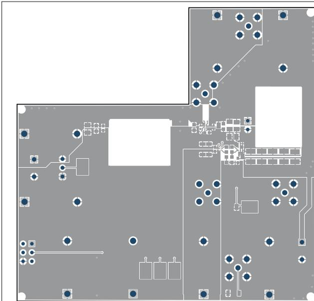
**Figure 4-5. Bottom Layer Routing**
