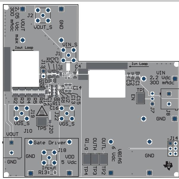
**Figure 4-6. Bottom Assembly Layer and Silk Screen**
