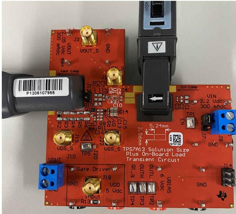
**Figure 3-2. TPS7A13EVM-057 With Current Probes Attached**
