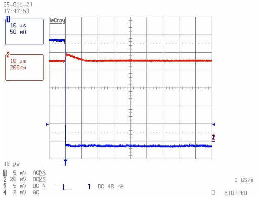
**Figure 3-4. TPS7A13EVM-057 Load Transient Results: 300-mA to 1-mA Load Step**
