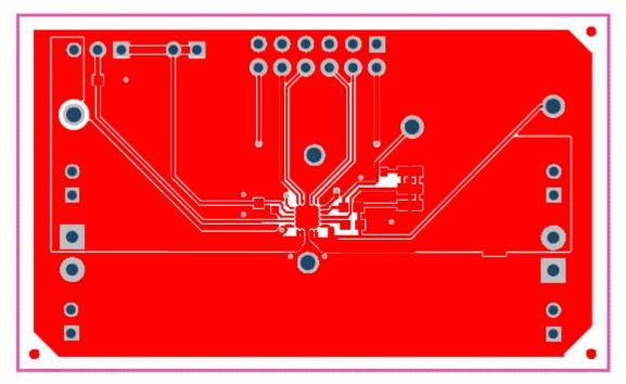
Figure 2. Top Layer Routing
