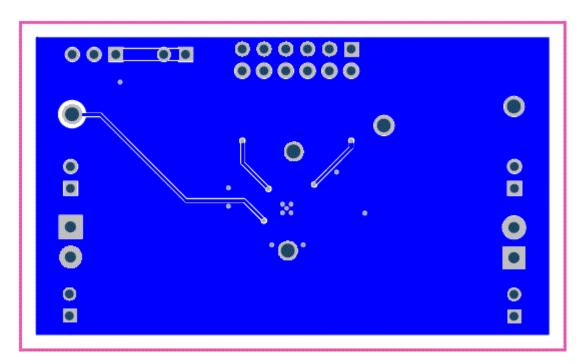
Figure 3. Bottom Layer Routing
