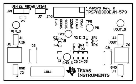
Figure 1. Assembly Layer
