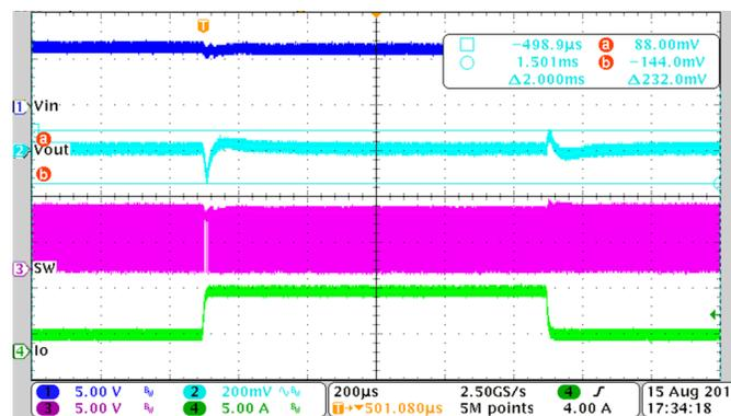
$V_{IN} = 6\text{ V}$ ,  $V_{OUT} = 4.95\text{ V}$ , Slew Rate =  $2.5\text{ A}/\mu\text{s}$
