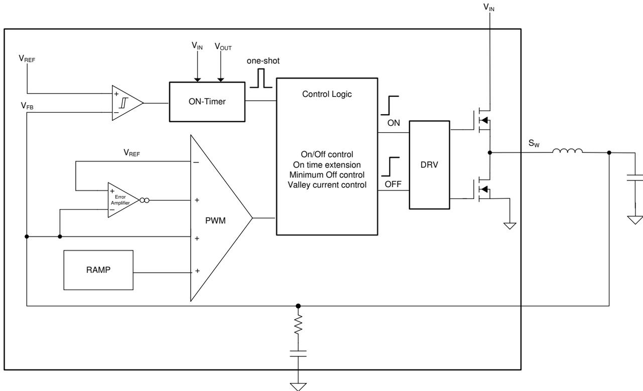
Figure 2. Detail D-CAP3™ Control Block Diagram in TPS568230
