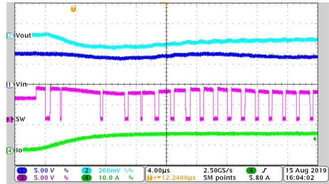
$V_{IN} = 6\text{ V}$ ,  $V_{OUT} = 4.95\text{ V}$ , Slew Rate =  $2.5\text{ A}/\mu\text{s}$
