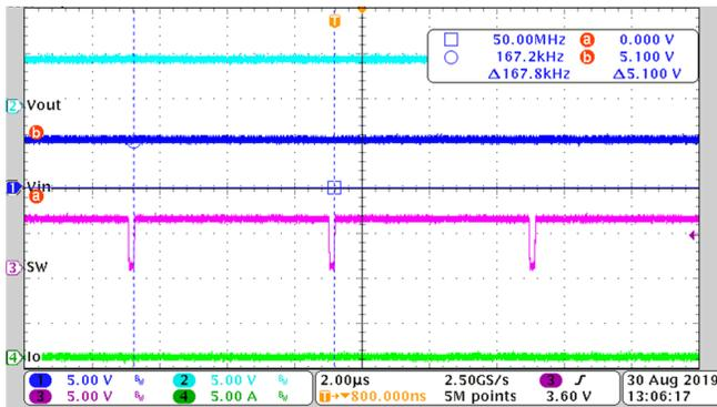
$V_{IN} = 5.1\text{ V}$ ,  $V_{OUT} = 4.95\text{ V}$ ,  $I_O = 0\text{ A}$
