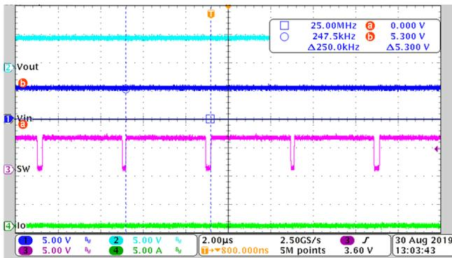
$V_{IN} = 5.3\text{ V}$ ,  $V_{OUT} = 4.95\text{ V}$ ,  $I_O = 0\text{ A}$
