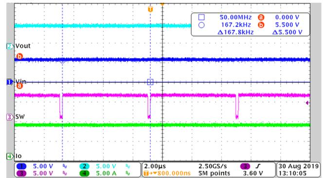
$V_{IN} = 5.5\text{ V}$ ,  $V_{OUT} = 4.95\text{ V}$ ,  $I_O = 8\text{ A}$
