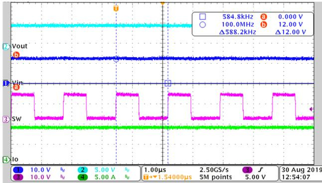
$V_{IN} = 12\text{ V}$ ,  $V_{OUT} = 4.95\text{ V}$ ,  $I_O = 8\text{ A}$
