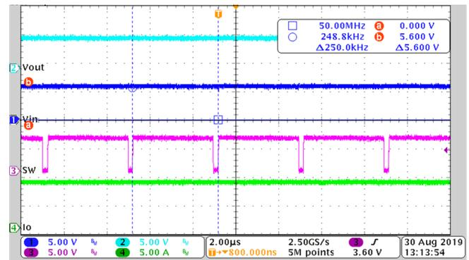
$V_{IN} = 5.6\text{ V}$ ,  $V_{OUT} = 4.95\text{ V}$ ,  $I_O = 8\text{ A}$
