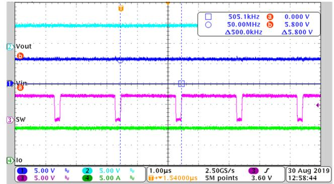
$V_{IN} = 5.8\text{ V}$ ,  $V_{OUT} = 4.95\text{ V}$ ,  $I_O = 8\text{ A}$
