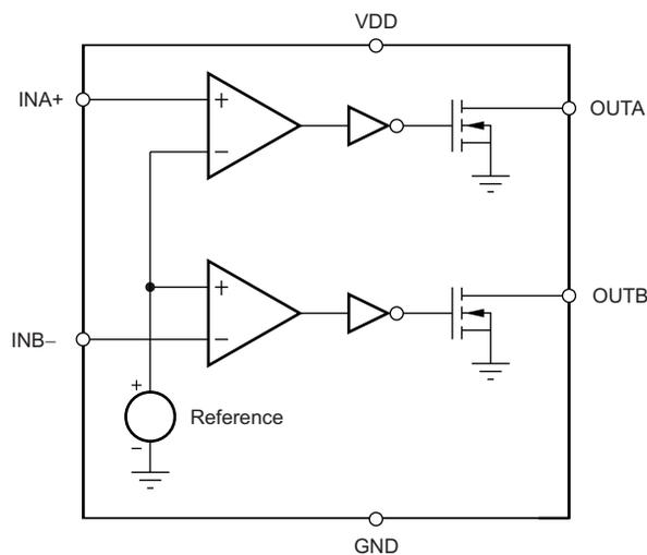
**Figure 2. TPS3700 Block Diagram**
