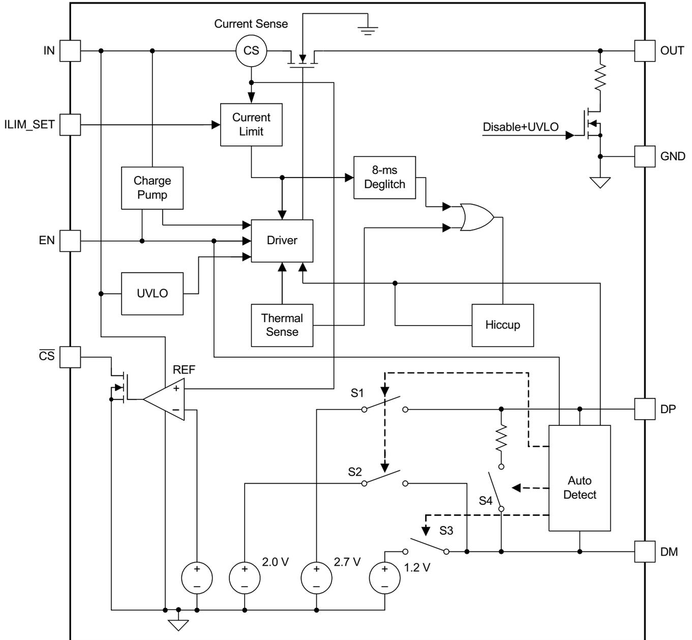
Figure 1. TPS2511 Block Diagram
