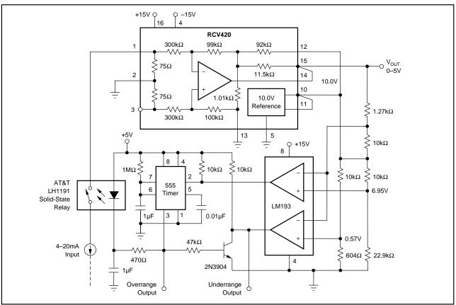
FIGURE 1. Input Protected RCV420.
