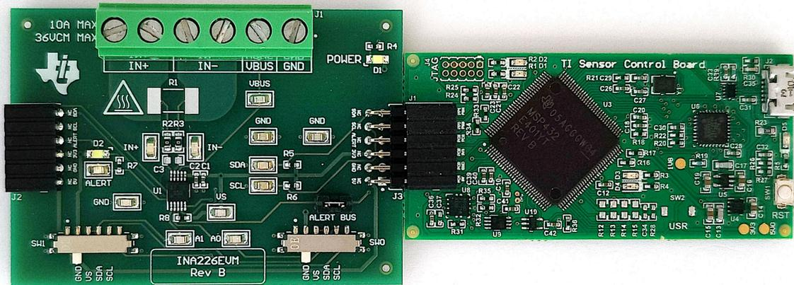
**Figure 4-1. EVM (Left) Connected to SCB Controller (Right)**
