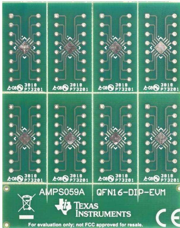
**Figure 1. QFN16-DIP-EVM**
