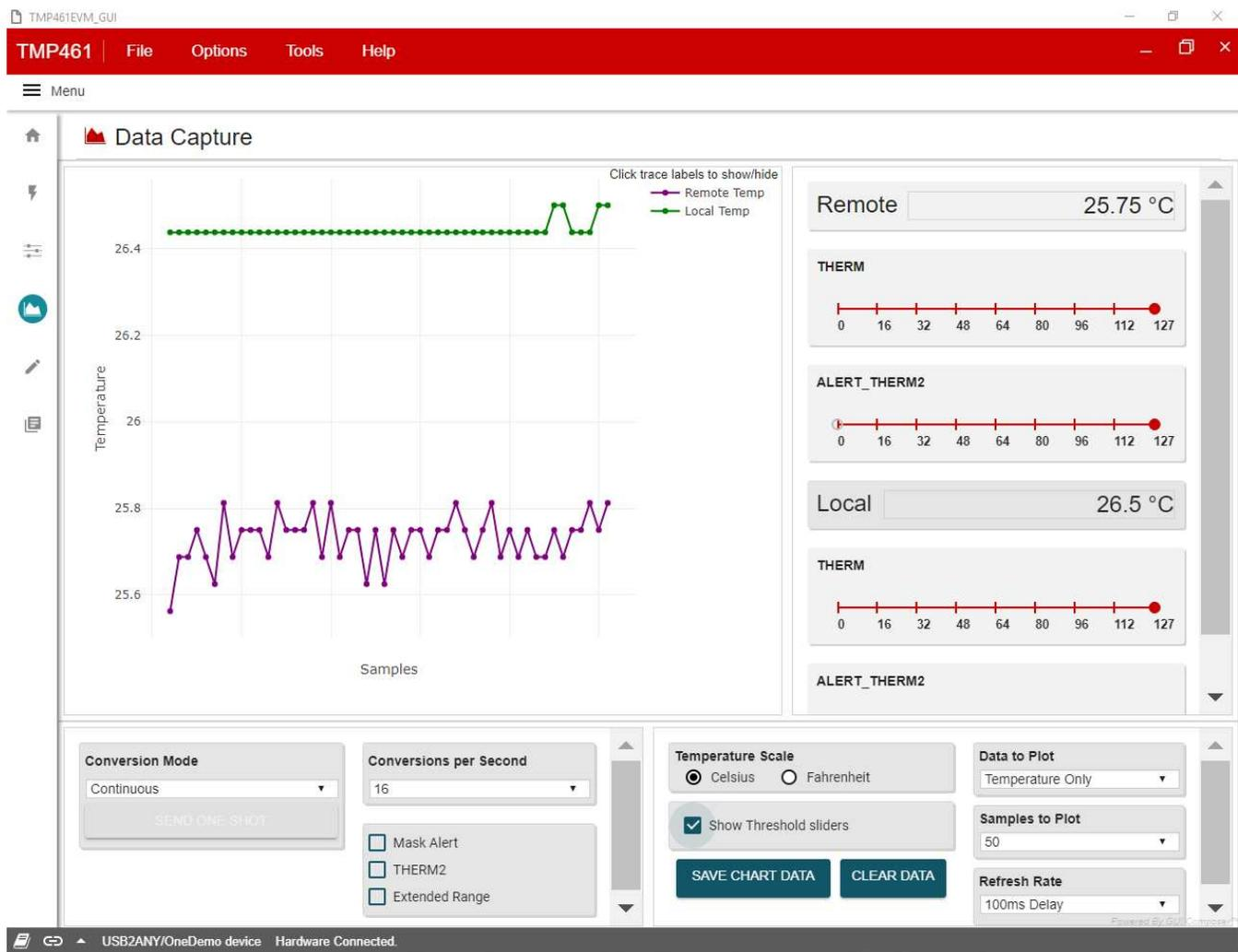
Figure 3-16. Threshold Sliders
