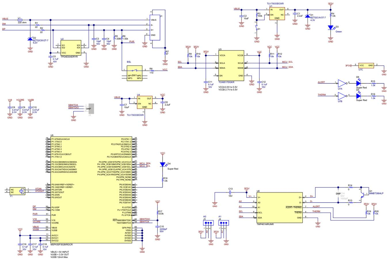
**Figure 4-1. TMP461EVM Schematic**
