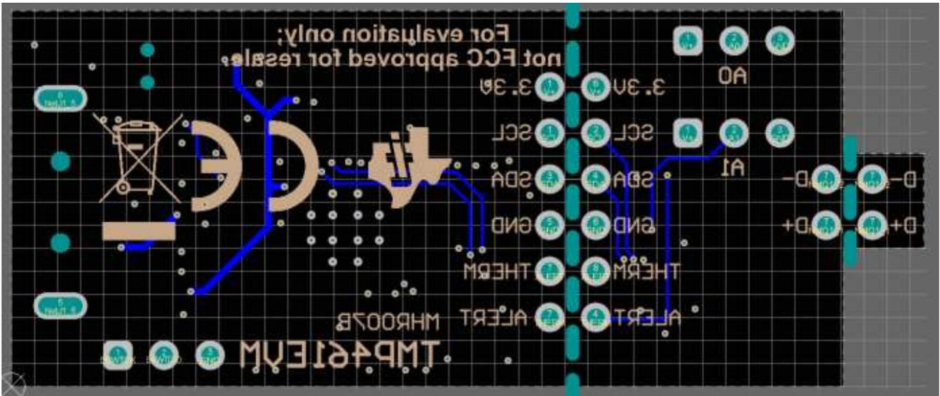
Figure 4-7. Bottom Assembly Layer
