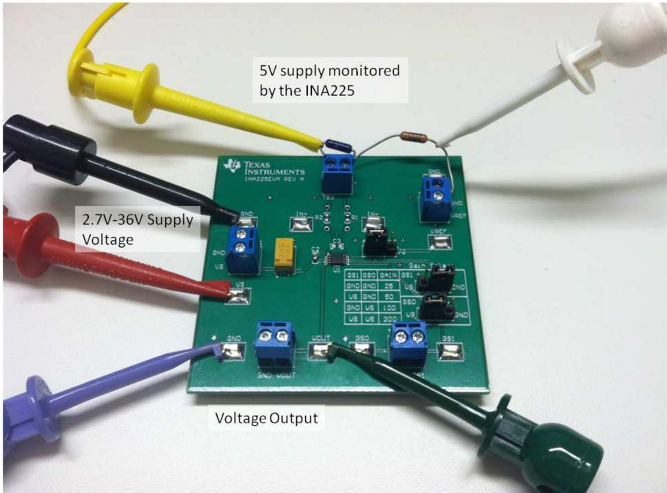
**Figure 5. Basic Setup of the INA225EVM**
