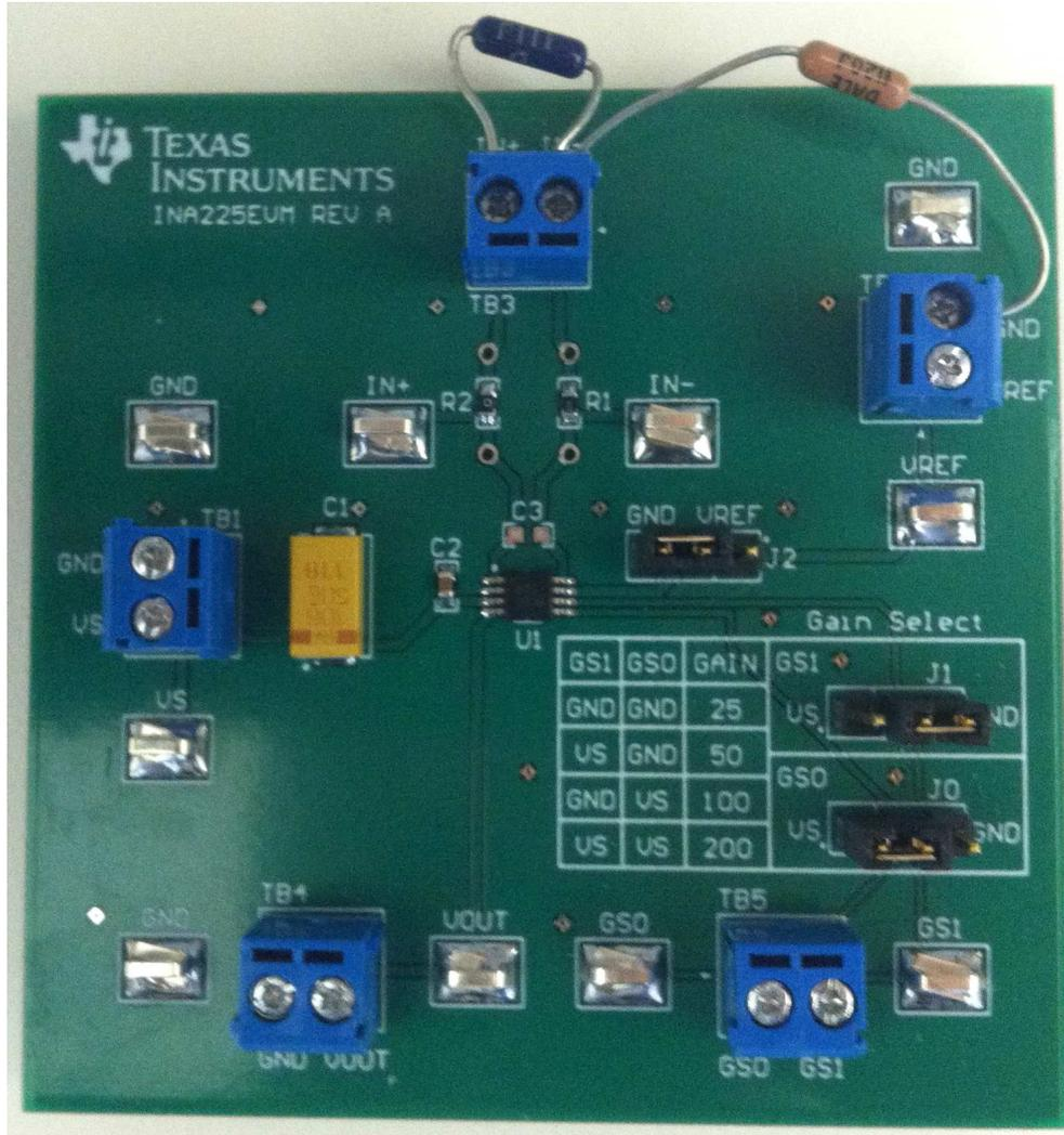
Figure 4. Basic Hardware Setup for the INA225EVM
