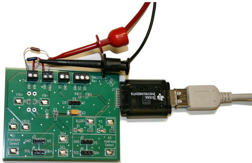
**Figure 3-1. Typical Hardware Test Connections for the INA231EVM**
