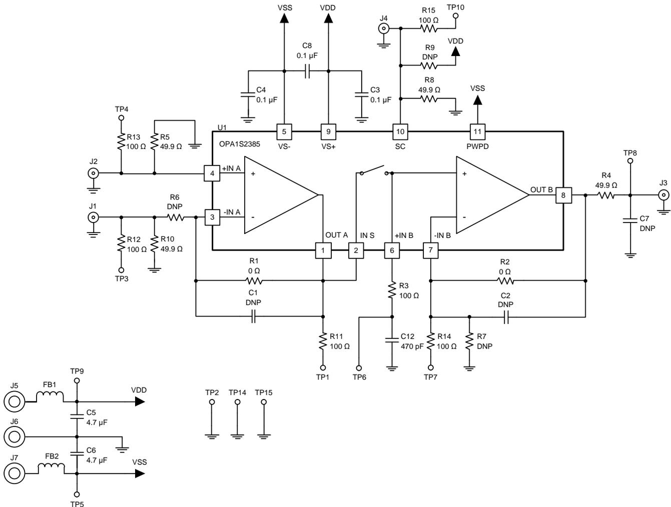
Figure 2. OPA1S238xEVM Schematic
