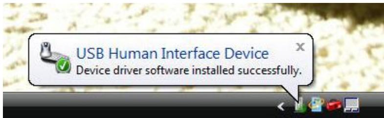
**Figure 3-3. Confirmation of SM-USB-DIG Platform Driver Installation**
