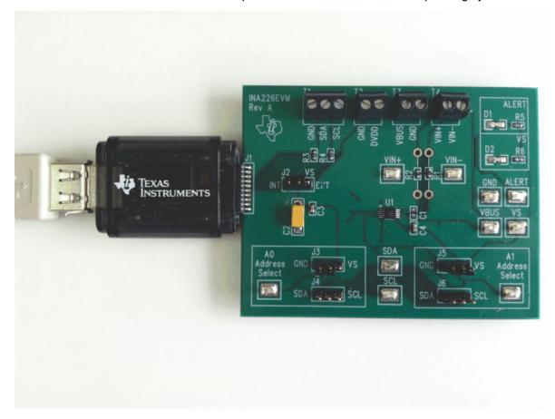
Figure 4-2. Connecting the USB Cable to the SM-USB-DIG Platform
