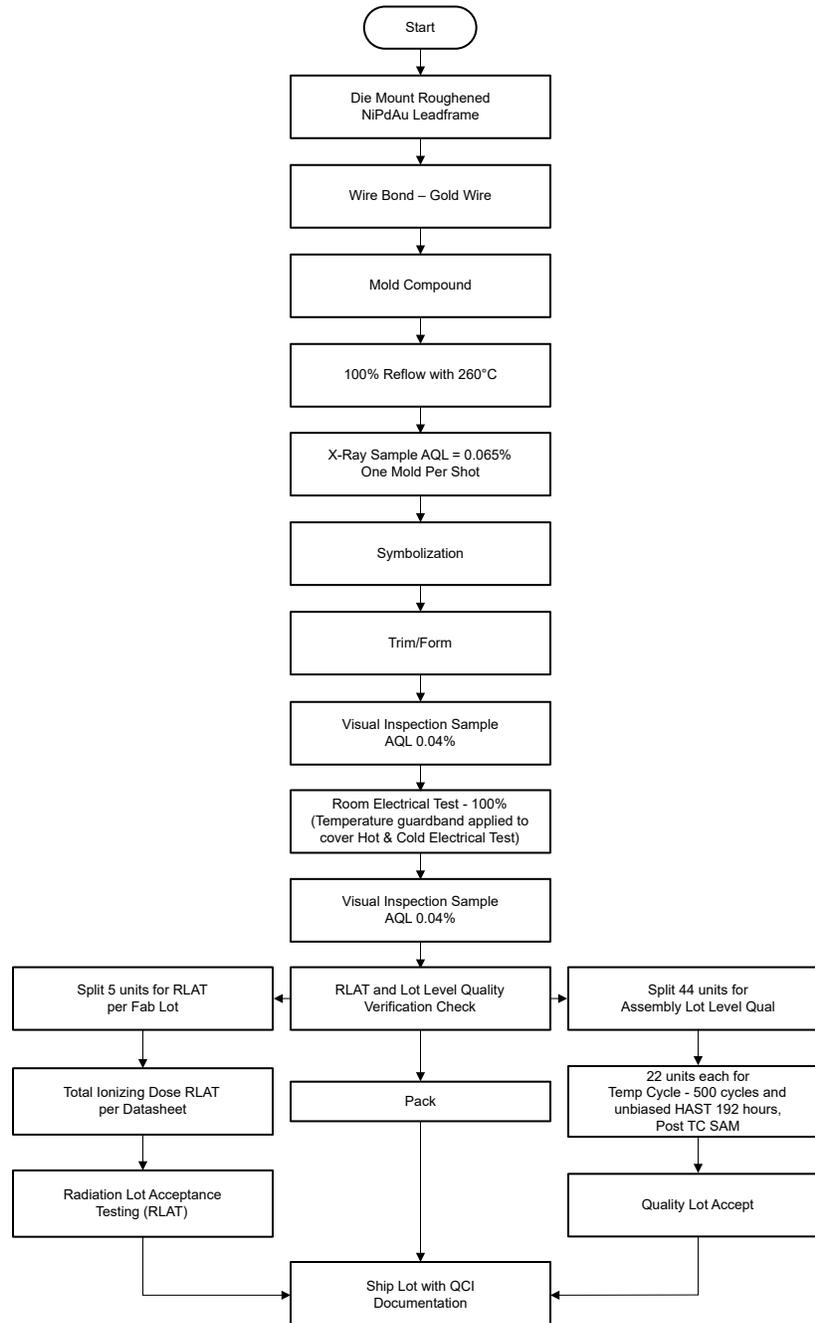
Figure 1-1. SN55LVTA4-SEP Space Enhanced Plastic Production Flow Chart
