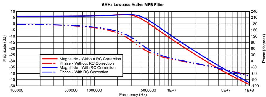
**Figure 3. 5MHz Low-Pass Active MFB Filter**
