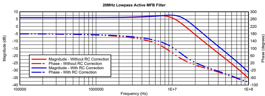
**Figure 4. 20MHz Low-Pass Active MFB Filter**
