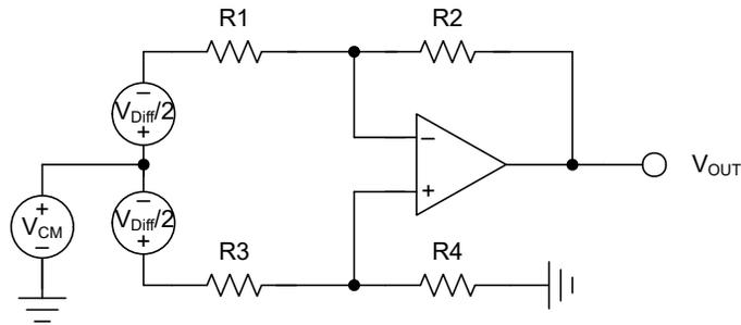
**Figure 4-2. Difference Amplifier With Differential and Common-Mode Input Signals**
