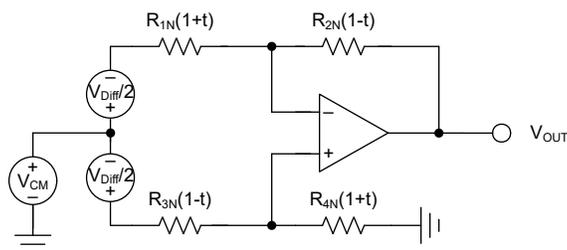
**Figure 5-1. Worst-Case Resistor Matching of Difference Amplifier Circuit**
