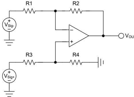
**Figure 2-1. Difference Amplifier Circuit**
