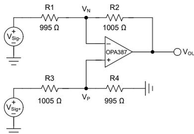
**Figure 2-3. Difference Amplifier with 0.5% Tolerance, 1-k $\Omega$  Resistors**
