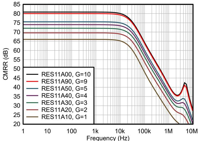
**Figure 3-3. Minimum CMRR of Difference Amplifier with Various RES11A-Q1 Gain Options, OPA387**
