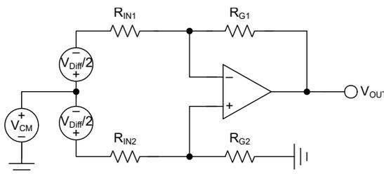
Figure 6-1. RES11A-Q1 Difference Amplifier Circuit
