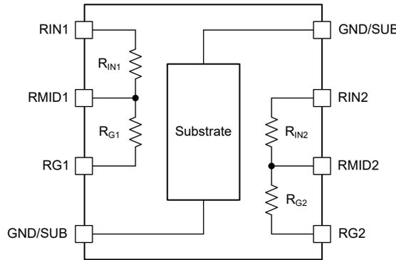
Figure 3-1. RES11A-Q1 Precision Matched Resistor Divider Pair
