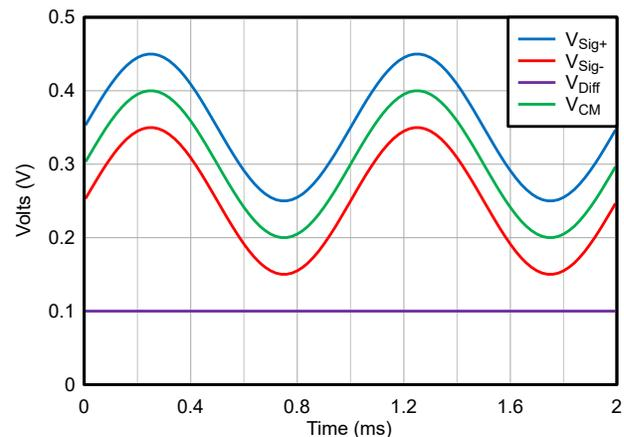
**Figure 1-2. DC Differential Signal with AC Common-Mode Voltage**
