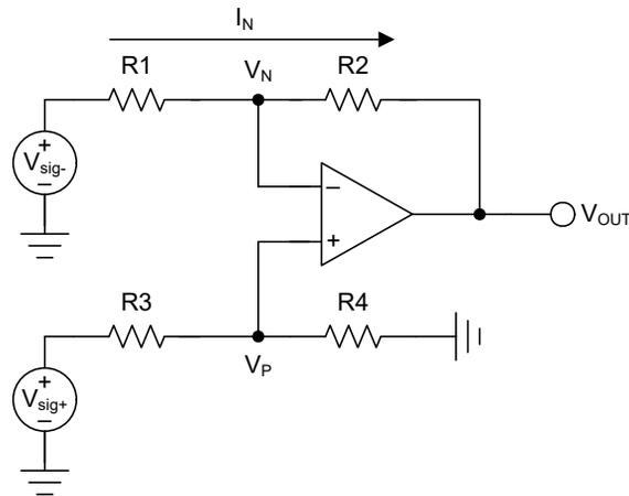
Figure 4-1. Difference Amplifier Circuit with Ideal Op-Amp
