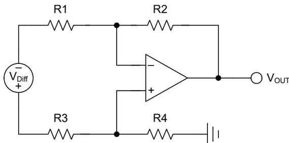
**Figure 4-3. Superposition: Differential-Mode**
