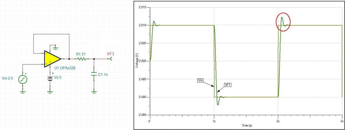
Figure 3-2. Transient Simulation of ADC Driver Using OPAx328
