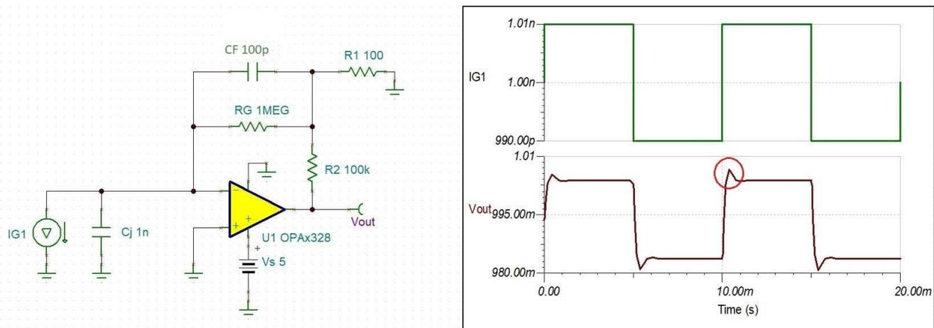
Figure 4-5. 1-GΩ TIA (in Noise Gain of 1000) Transient Stability Using OPAx328
