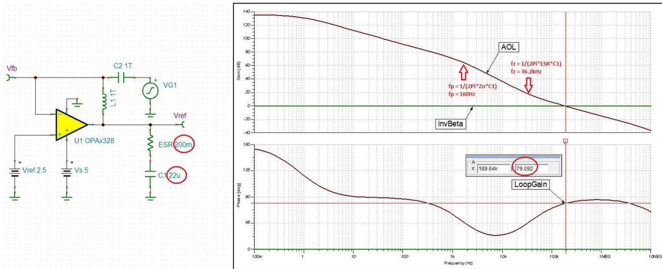
**Figure 2-1. Stability Analysis of Reference Buffering Using OPAx328**
