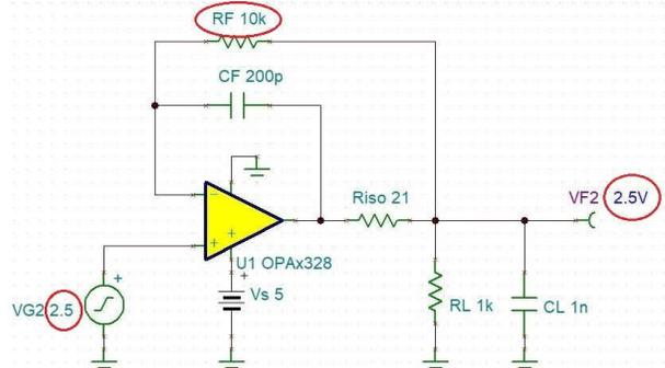
Figure 3-4. ADC Driver Dual Feedback Using OPAx328
