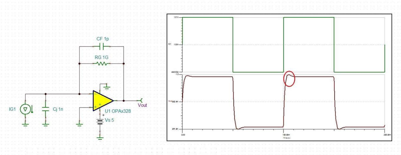
Figure 4-3. 1-GΩ TIA Transient Stability Using OPAx328
