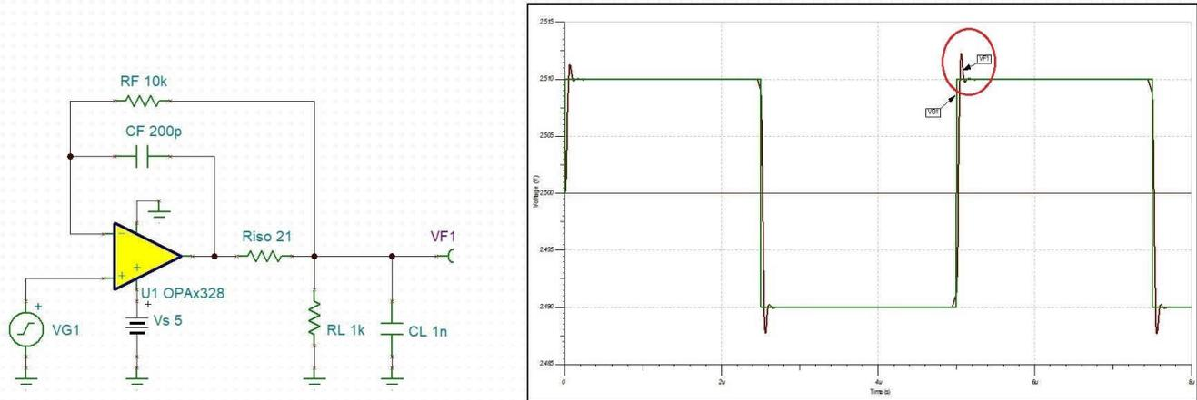
Figure 3-6. Dual Feedback ADC Driver Transient Simulation Using OPAX328
