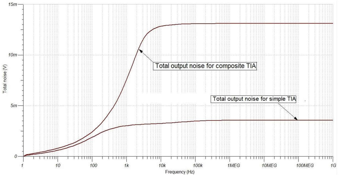
**Figure 4-6. Effect of 1-GΩ TIA Implementation on the Total Output Noise**
