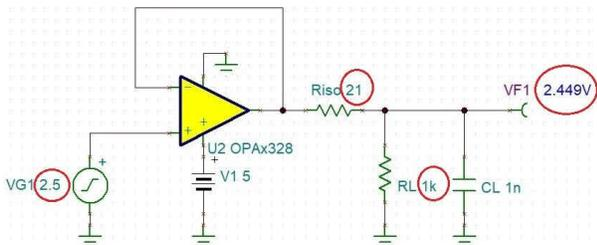
Figure 3-3. ADC Driver Gain Error Due to Resistive Loading
