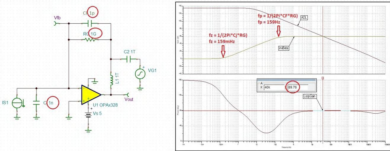
Figure 4-2. 1-GΩ TIA AC Stability Using OPAx328
