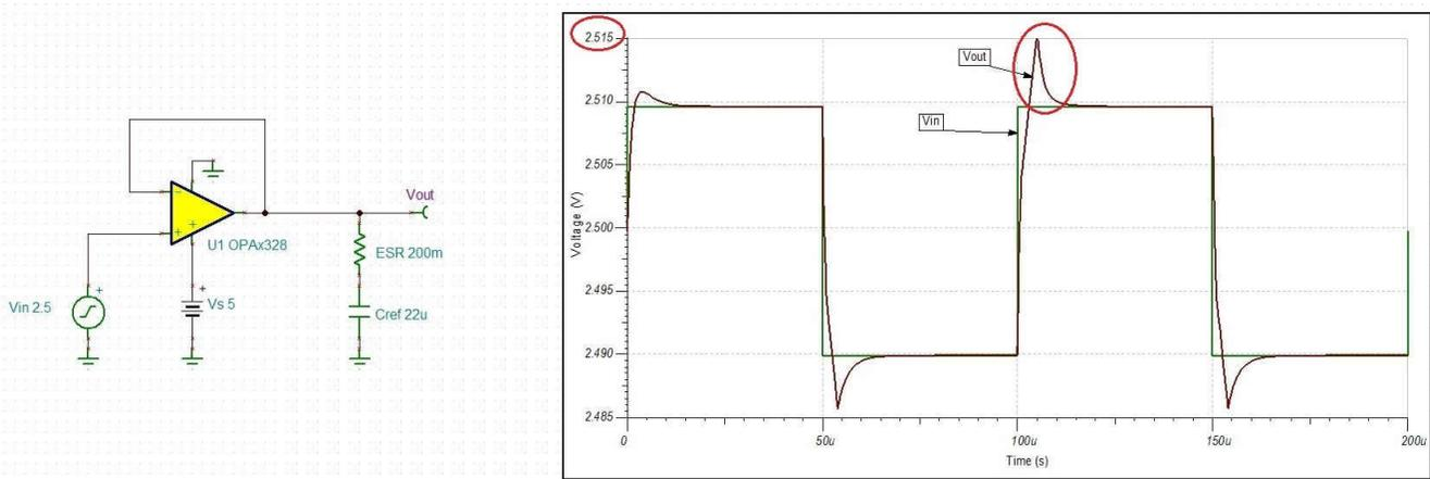
Figure 2-2. Transient Simulation of Reference Buffering Using OPAx328
