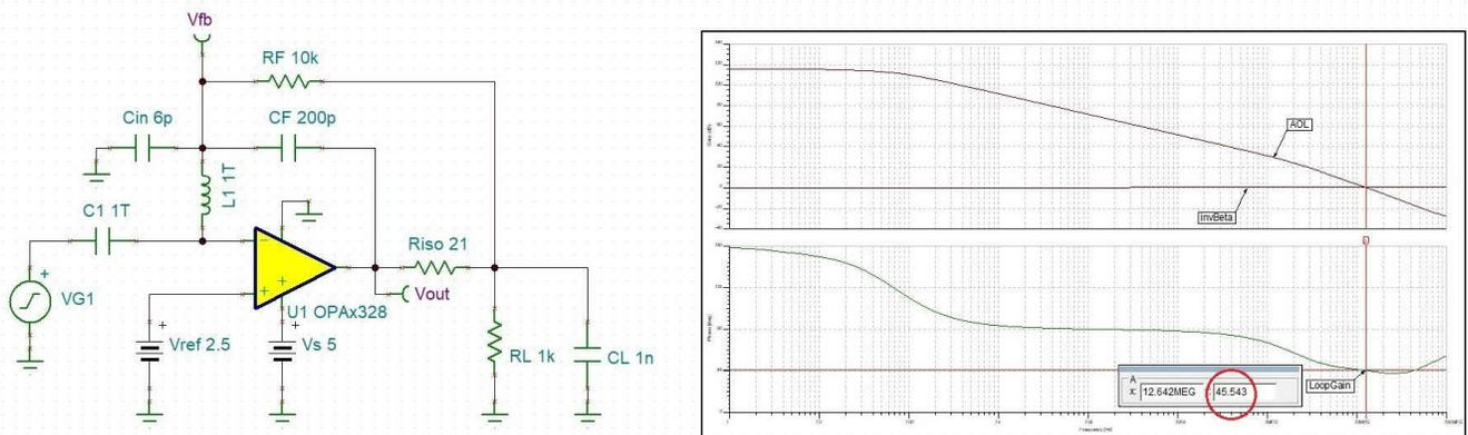
Figure 3-5. Dual Feedback ADC Driver Stability Analysis Using OPAx328
