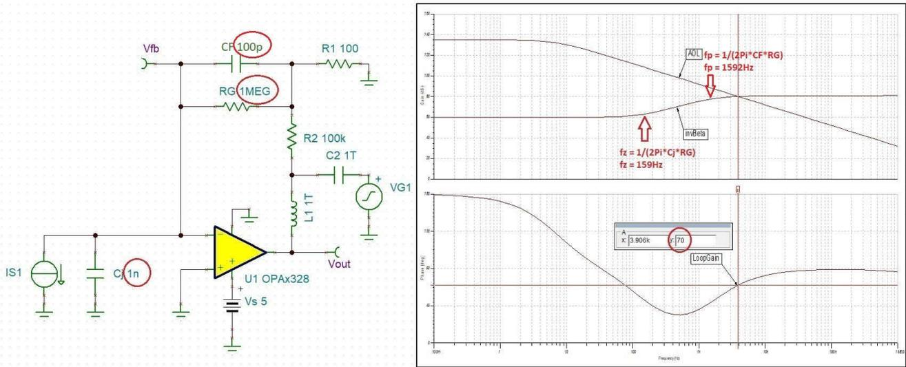
Figure 4-4. 1-GΩ TIA in Noise Gain of 1000 AC Stability Using OPAx328
