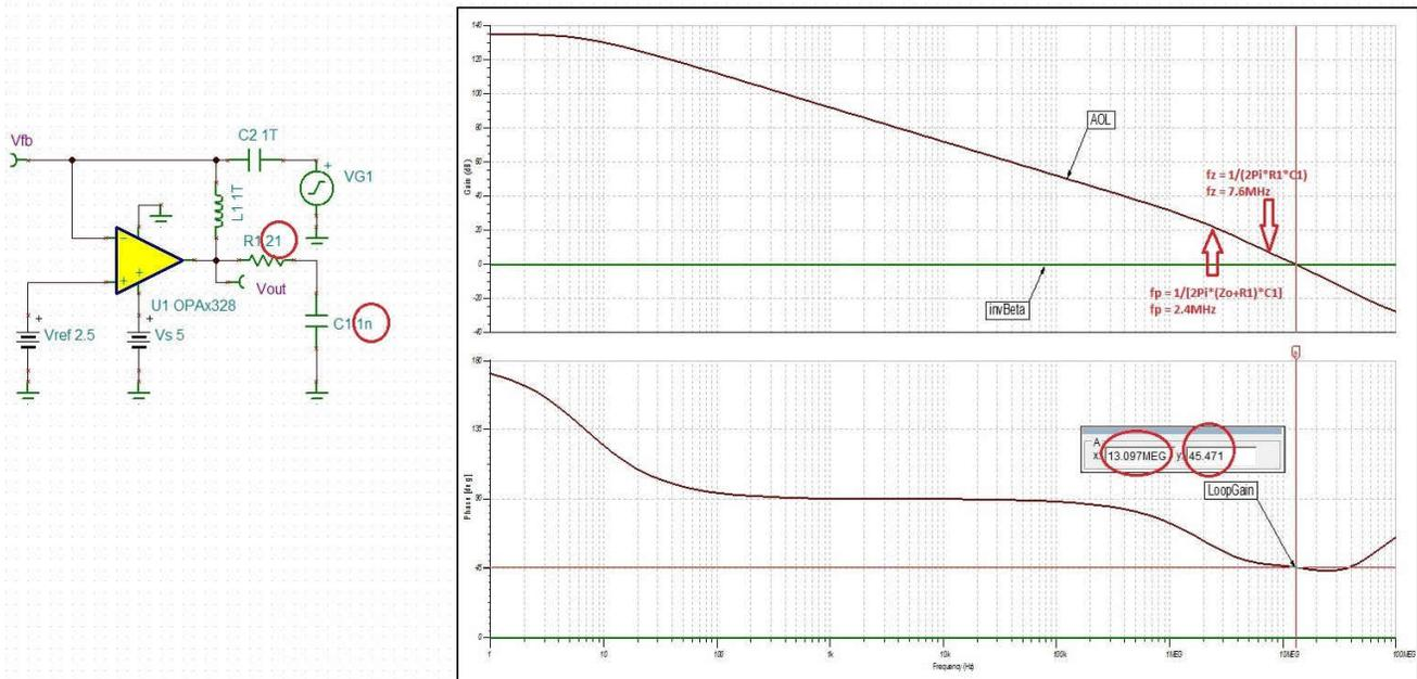
**Figure 3-1. Stability Analysis of ADC Driver Using OPAx328**
