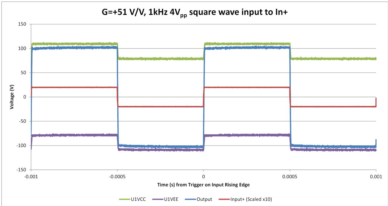
Figure A-10. Noninverting Configuration,  $G = +51 \text{ V/V}$ , 1-kHz Square Wave (Output 211  $V_{pp}$ )
