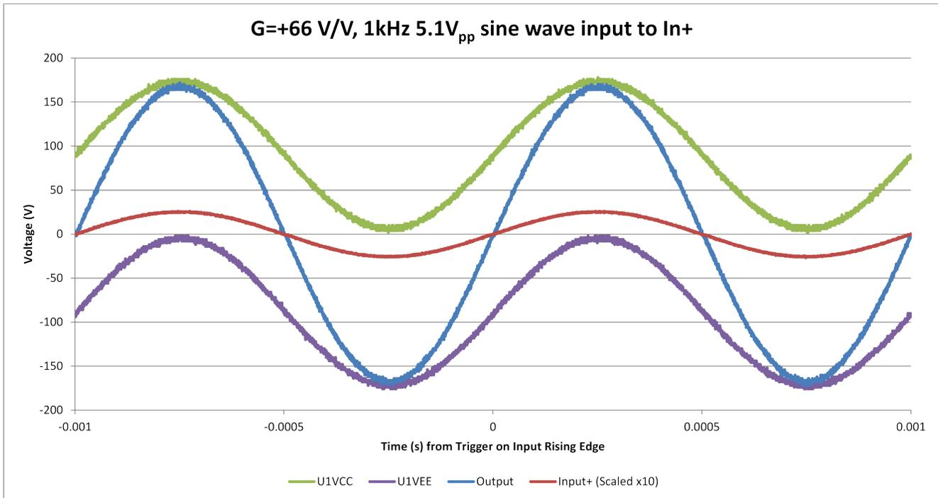
Figure A-4. Noninverting Configuration,  $G = +66 \text{ V/V}$ , 1-kHz Sine Wave (Output  $344 \text{ V}_{pp}$ )
