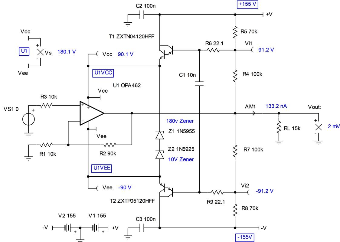
Figure 4-2. Darlington Transistor Supply-Rail Drivers for OPA462, 310-V Total Supply
