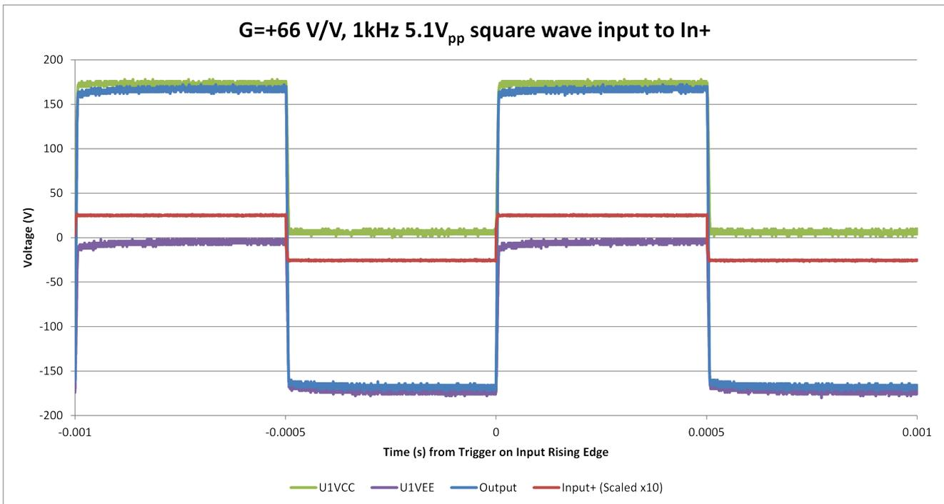
Figure A-5. Noninverting Configuration,  $G = +66 \text{ V/V}$ , 1-kHz Square Wave (Output  $344 \text{ V}_{pp}$ )
