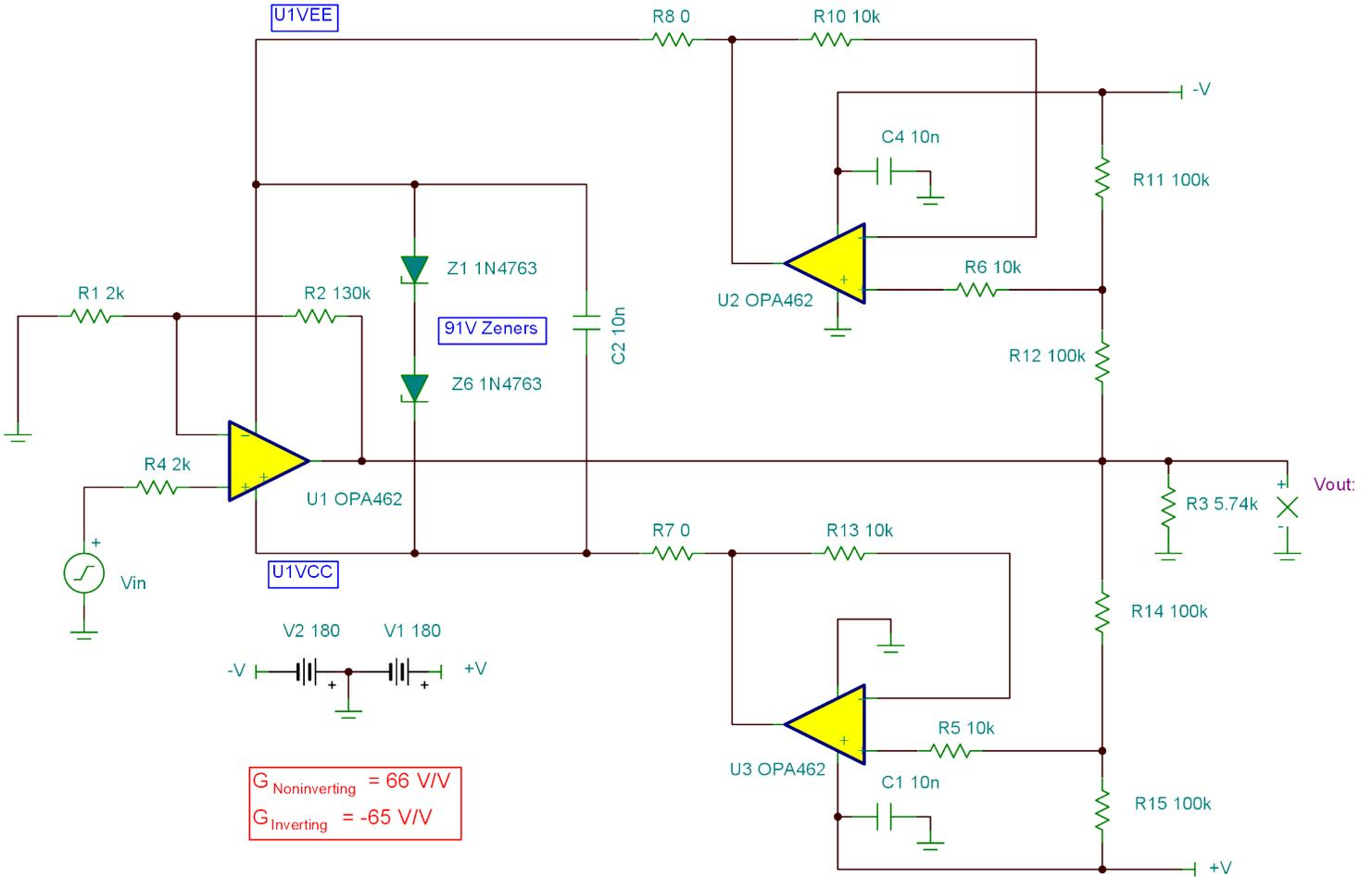
Figure A-3. Three OPA462 Three op amp Solution Schematic
