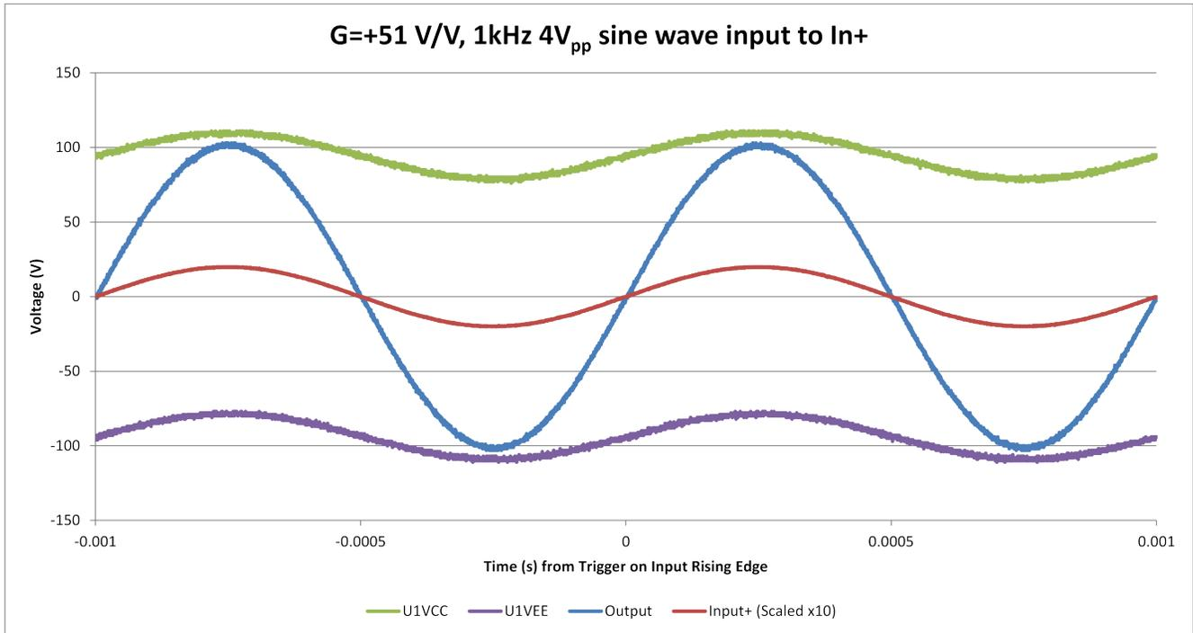
Figure A-9. Noninverting Configuration,  $G = +51 \text{ V/V}$ , 1-kHz Sine Wave (Output 206  $V_{pp}$ )
