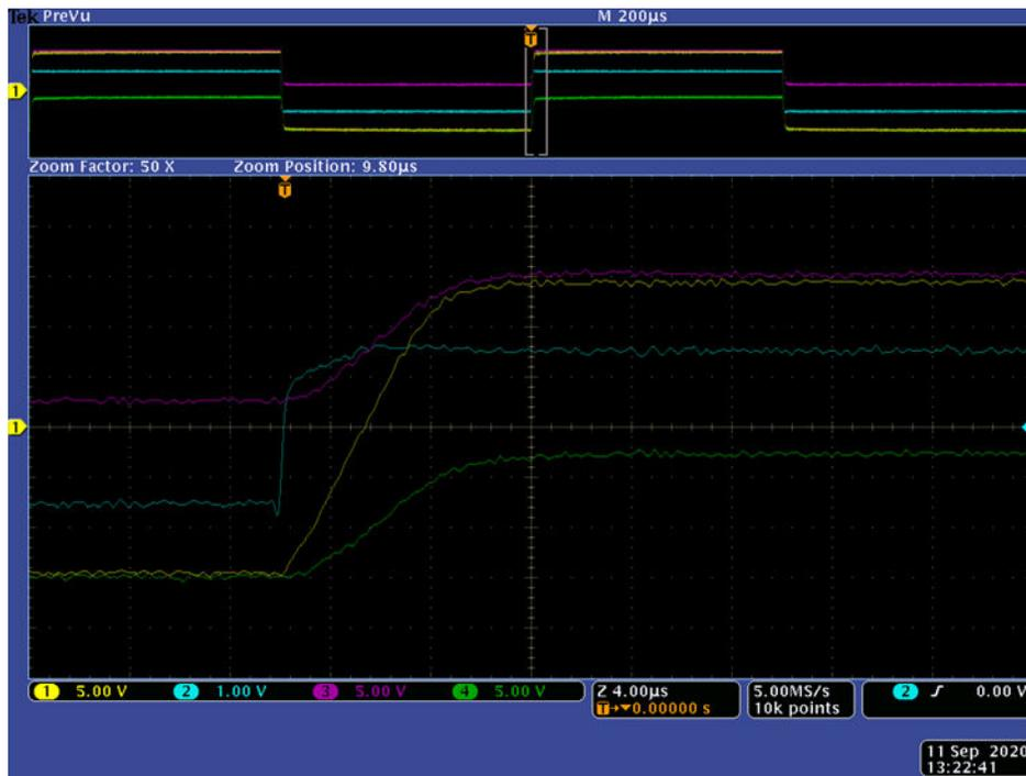
Figure A-17. Noninverting Configuration,  $G = +96.5 \text{ V/V}$ , 1-kHz Square Wave ( $3.08 \text{ V}_{pp}$ ), Zoom on Rising Edge
