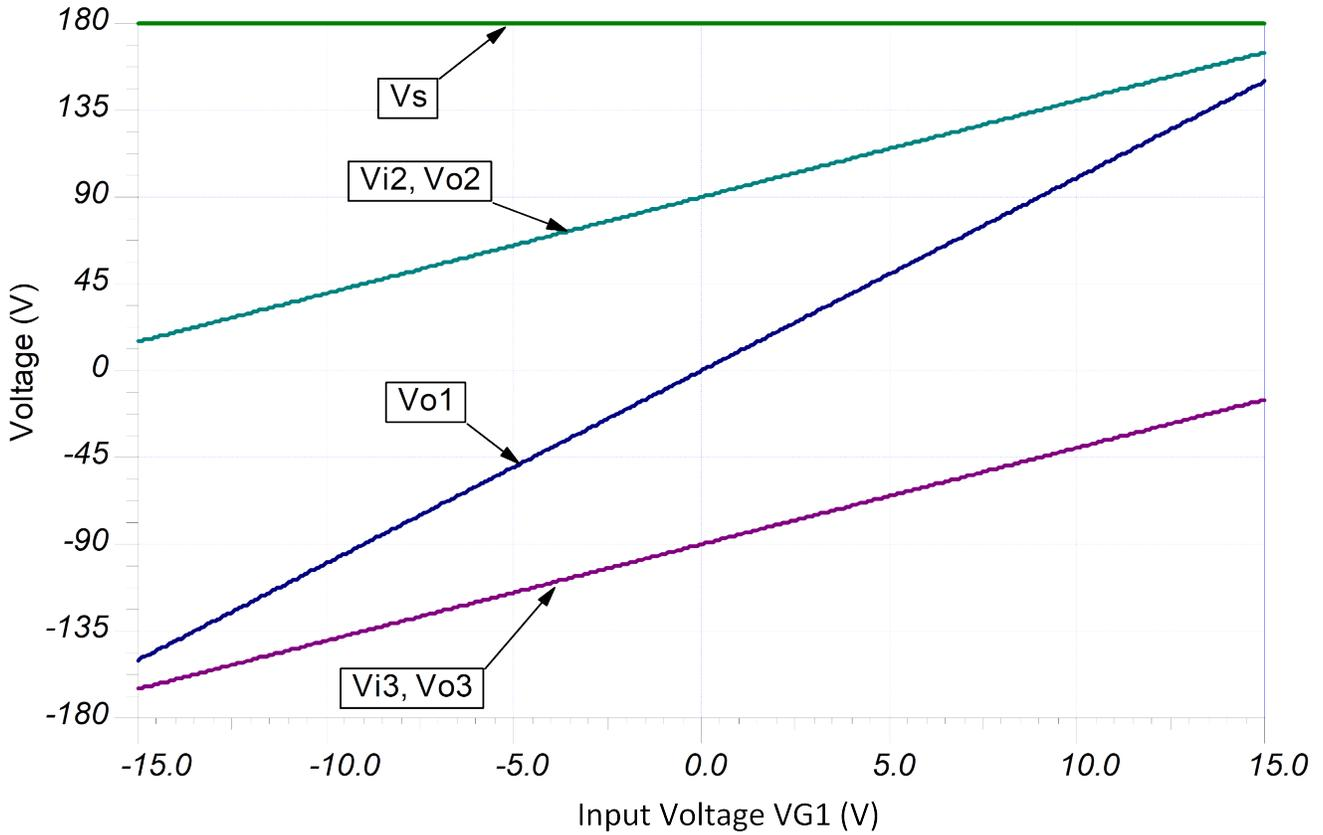
**Figure 2-3. Circuit Voltages for the Three OPA462 HV Solutions as the DC Input Voltage  $V_{G1}$  is Swept From -15 V to +15 V**
