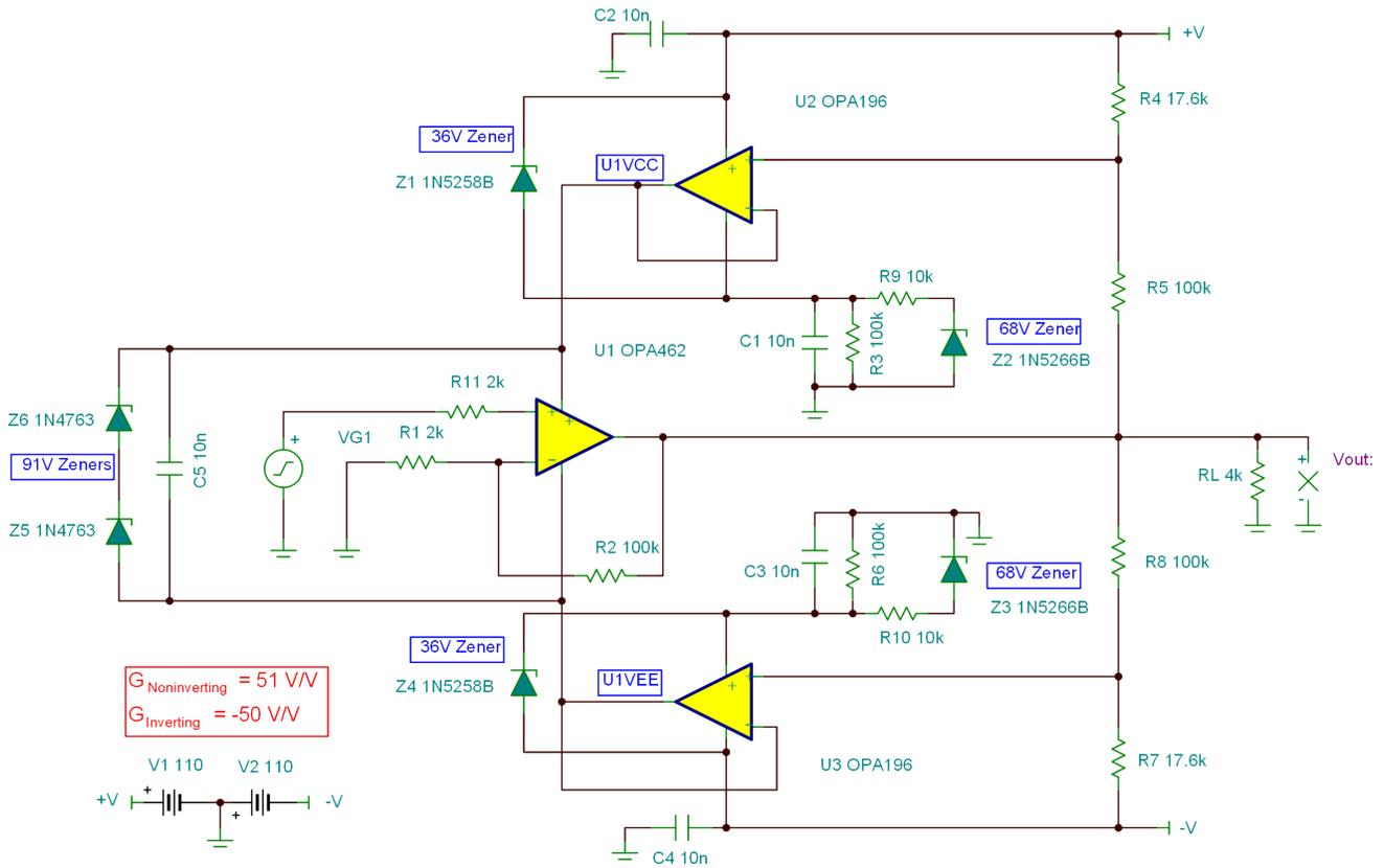
Figure A-8. Lower Voltage, Lower Cost Three Op-amp Solution
