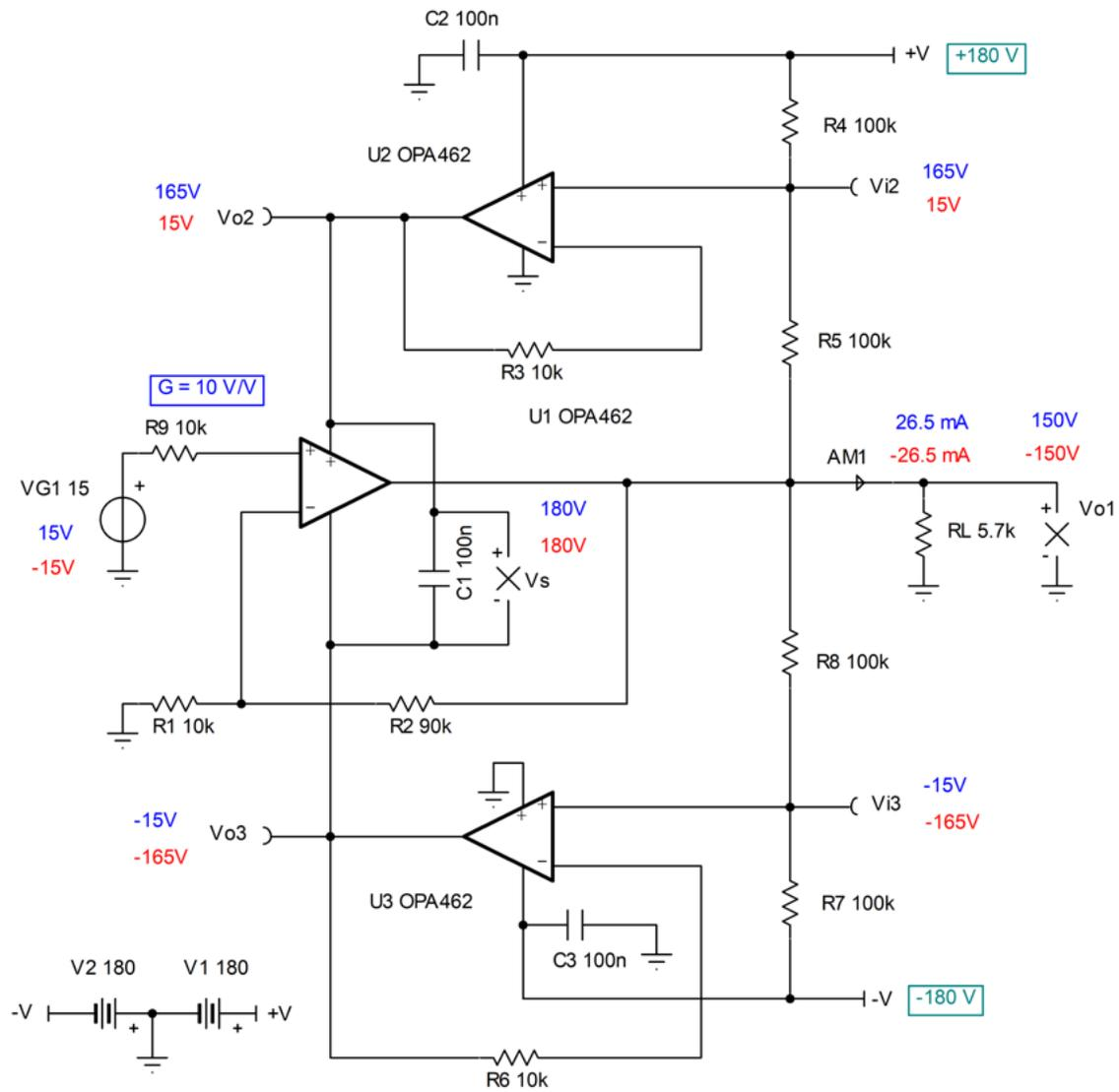
Figure 2-2. Three OPA462 HV Solution With DC Input Voltages of +15 V (Blue) and -15 V (Red)
