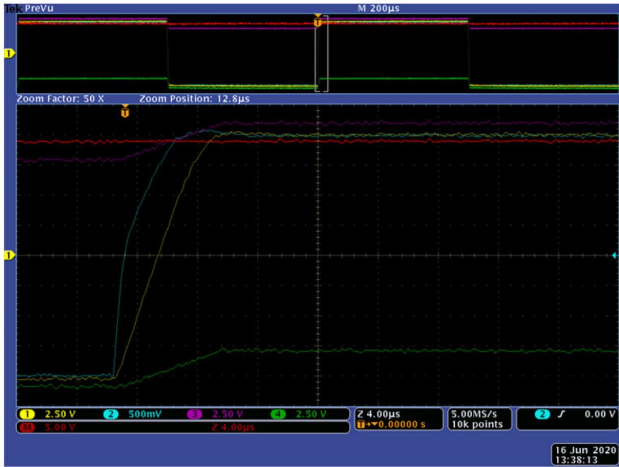
Figure A-12. Noninverting Configuration  $G = +51 \text{ V/V}$ , 1-kHz Square Wave ( $4 \text{ V}_{pp}$ ), Zoom on Rising Edge
