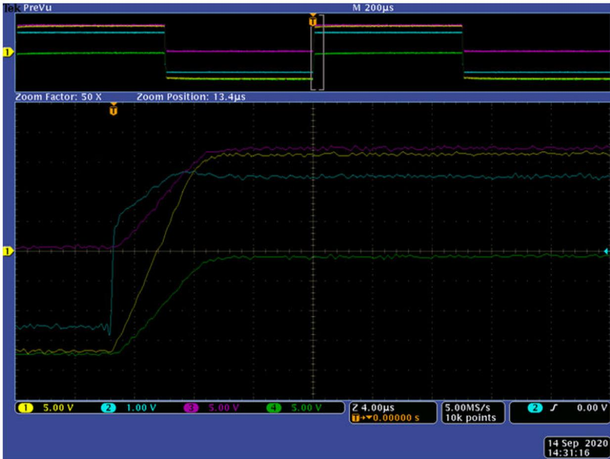
Figure A-7. Noninverting Configuration,  $G = +66 \text{ V/V}$ , 1-kHz Square Wave ( $5.1 \text{ V}_{pp}$ ), Zoom on Rising Edge
