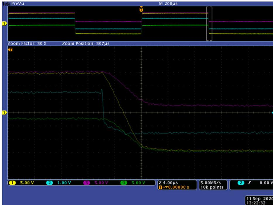
Figure A-16. Noninverting Configuration,  $G = +96.5 \text{ V/V}$ , 1-kHz Square Wave ( $3.08 \text{ V}_{pp}$ ), Zoom on Falling Edge
