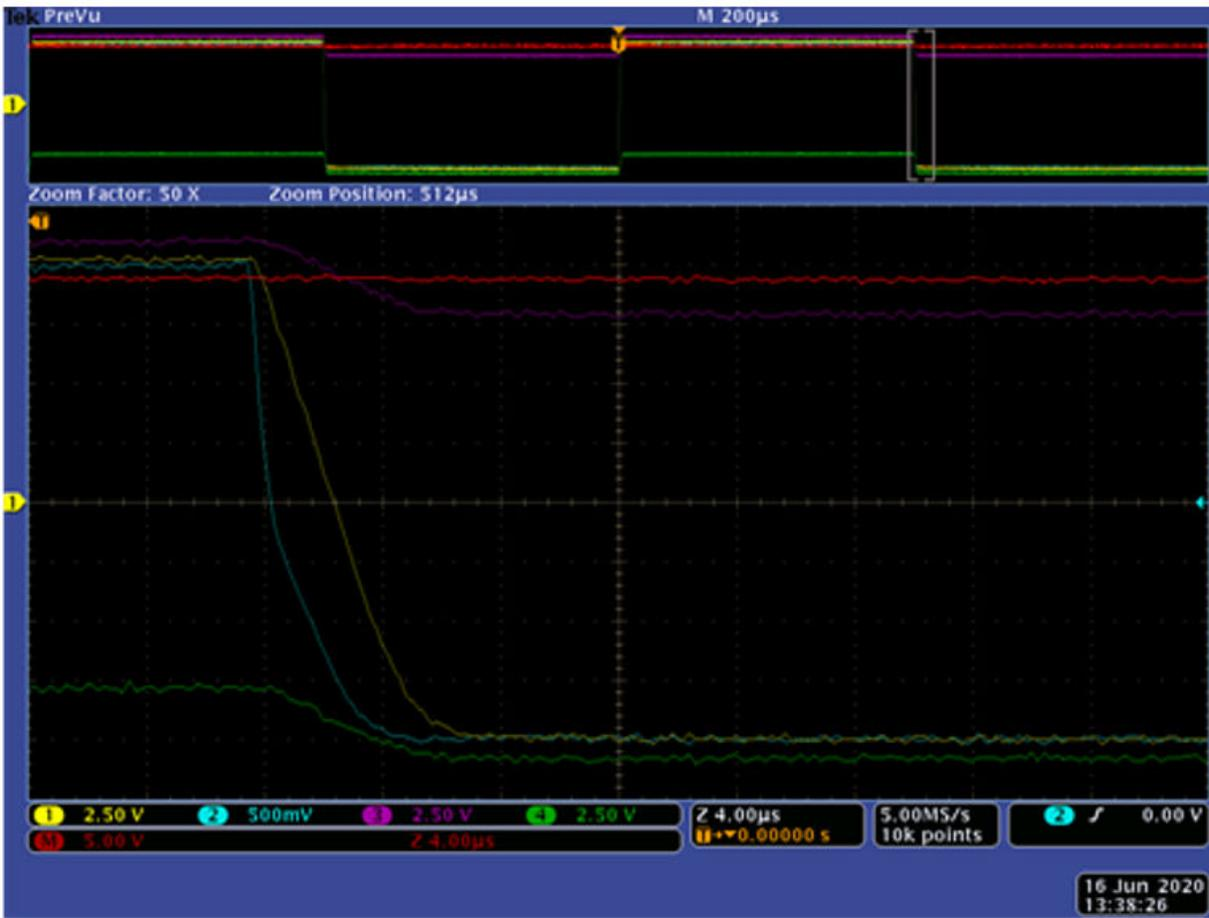
Figure A-11. Noninverting Configuration,  $G = +51 \text{ V/V}$ , 1-kHz Square Wave ( $4 \text{ V}_{pp}$ ), Zoom on Falling Edge
