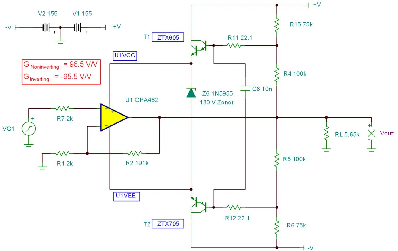
Figure A-13. OPA462 300 V<sub>pp</sub> Output Solution With Discrete Transistor Supply-Rail Drivers
