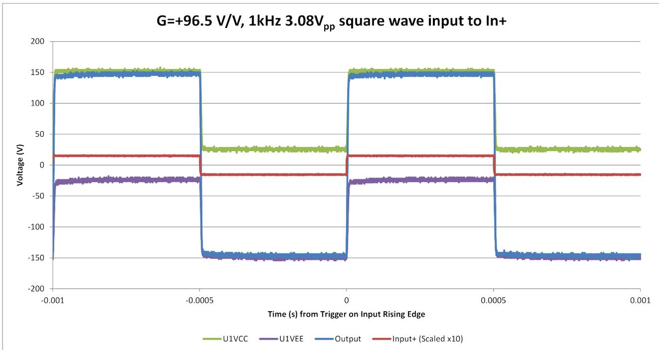
Figure A-15. Noninverting Configuration,  $G = +96.5 \text{ V/V}$ , 1-kHz Square Wave (Output  $304 \text{ V}_{pp}$ )
