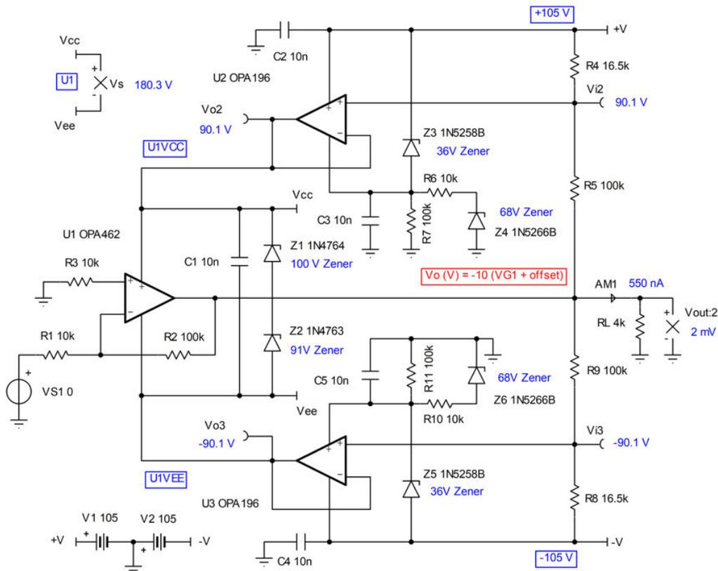
Figure 3-1. 200 V<sub>pp</sub> Output Solution Achieved by Applying Lower Voltage Op Amps at the U2 and U3 Positions
