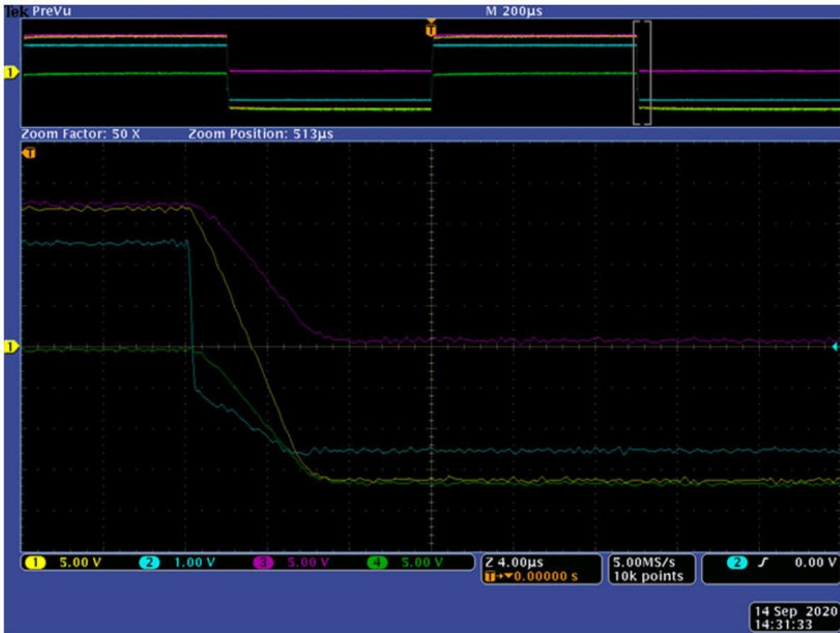
Figure A-6. Noninverting Configuration,  $G = 66 \text{ V/V}$ , 1-kHz Square Wave ( $5.1 \text{ V}_{pp}$ ), Zoom on Falling Edge
