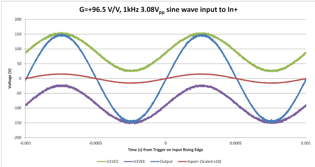
Figure A-14. Noninverting Configuration,  $G = +96.5 \text{ V/V}$ , 1 kHz Sine Wave (Output  $298 \text{ V}_{pp}$ )
