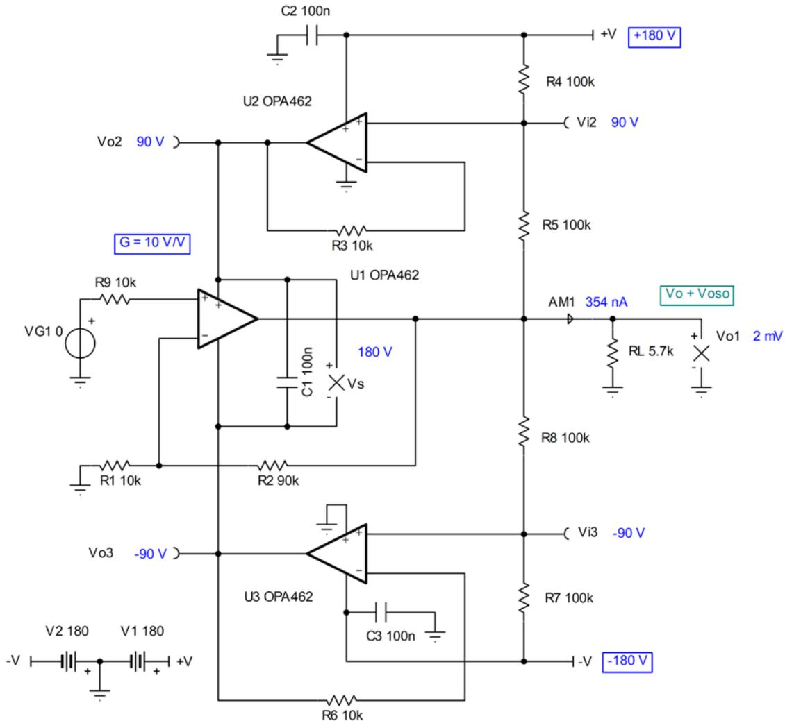
Figure 2-1. Three OPA462 Op Amp HV Solution
