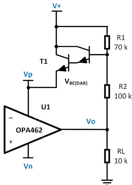
Figure 4-1. Darlington Transistor Driver for U1 OPA462 Positive Supply pin
