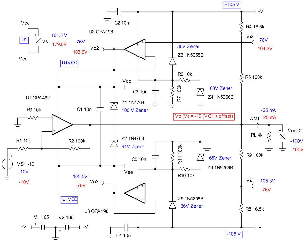
**Figure 3-2. OPA462 HV + OPA196 Solution With Input Voltages of +10 V (Blue) and -10 V (Red)**
