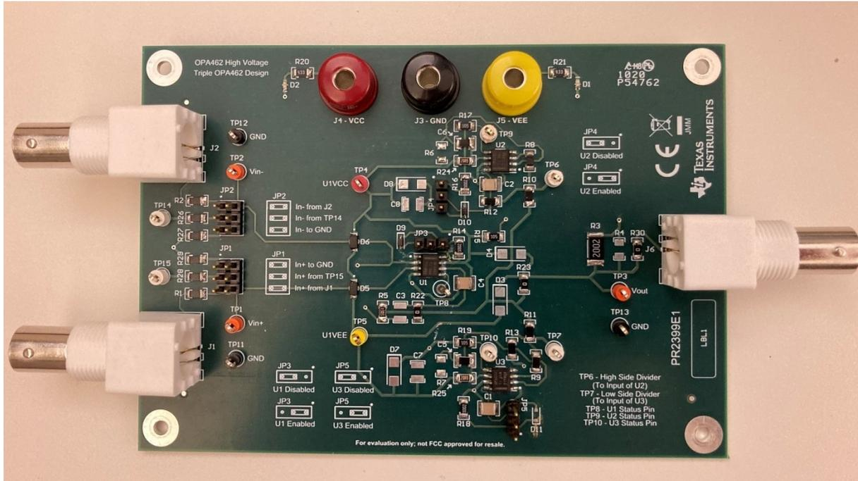
**Figure A-2. Example Test PCB Development for OPA462 Three Op Amp Rail Drivers Circuit**
