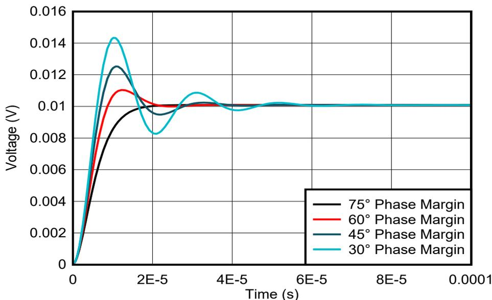
Figure 5-1. Small-Signal Step Response and Phase Margin
