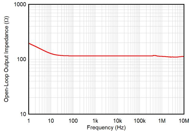
**Figure 1-1. Open-Loop Output Impedance vs Frequency, OPA392**
