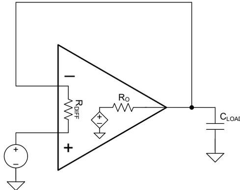
**Figure 4-1. Op Amp Output Resistance Internal Model**
