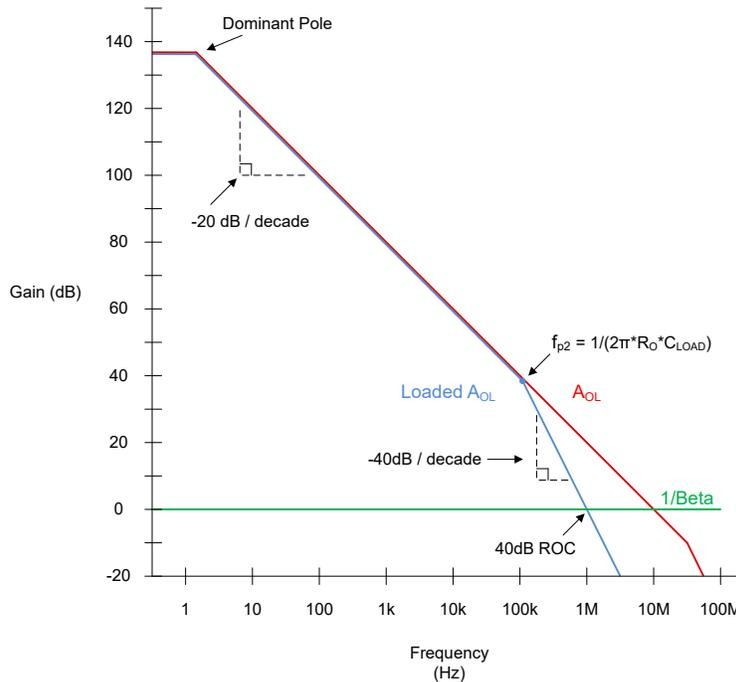
**Figure 4-2. Effects of Capacitive Load on Amplifier Open-Loop Gain**
