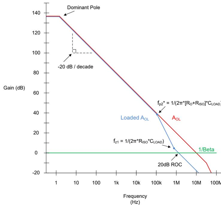
**Figure 4-4. Effects of R<sub>ISO</sub> on Amplifier Open-Loop Gain with Capacitive Load**
