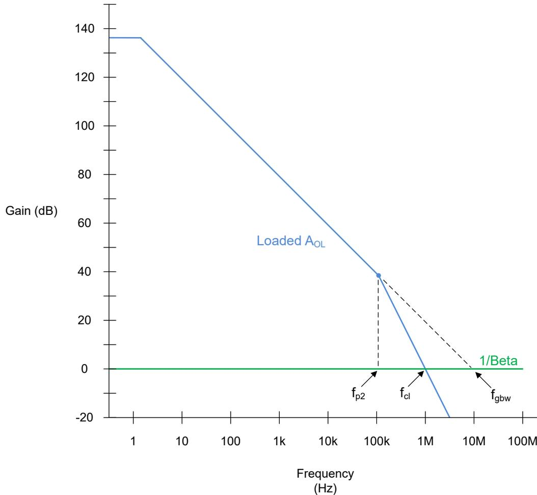
**Figure 5-2. Amplifier Open-Loop Gain with Capacitive Loading**
