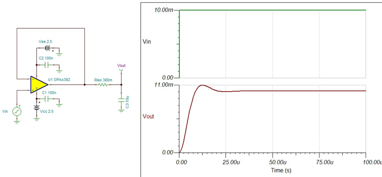
**Figure 3-2. Stable Buffer Configuration with Optimal R<sub>ISO</sub>**
