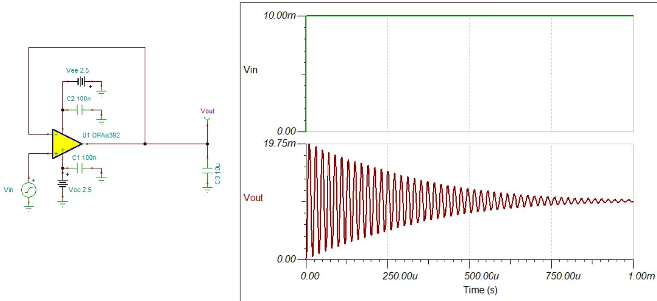
Figure 3-1. Unstable Buffer Configuration, 10  $\mu\text{F}$  Load
