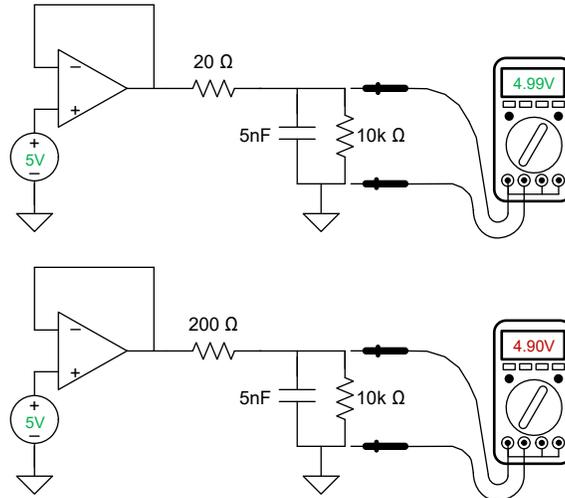
Figure 4-5.  $R_{ISO}$  Voltage Divider with Resistive-Capacitive Load
