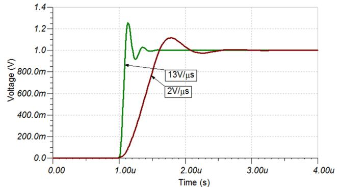
**Figure 3. Slew Rate Comparison**
