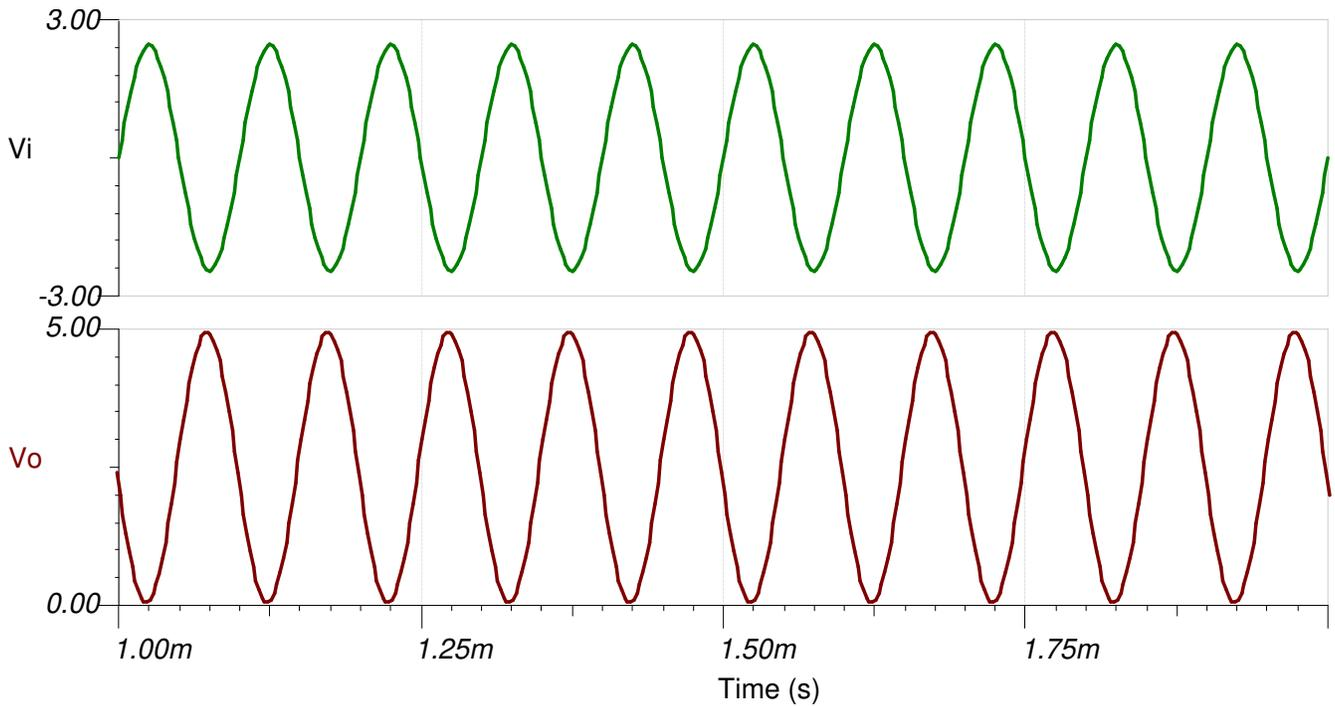
Filter Output in Response to a 5-V<sub>pp</sub>, 10-kHz Input-Signal (Gain = -1V/V).
