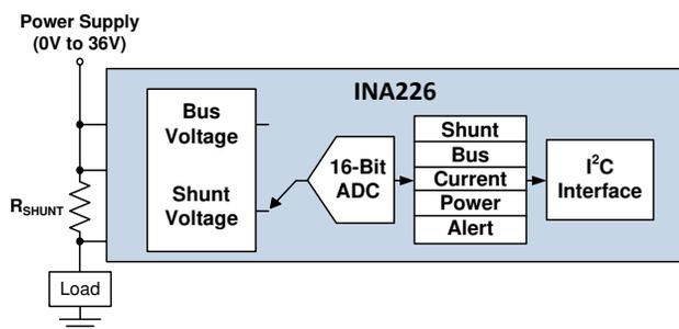
**Figure 2. INA226, Precision Current, Voltage, Power Sensing ADC**
