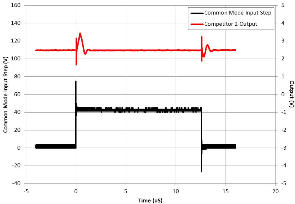
**Figure 7. Competitor 2 Output vs 40-V Common-Mode Step Input**
