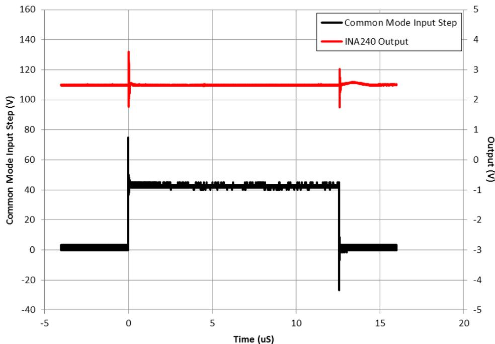
**Figure 5. INA240 Output vs 40-V Common-Mode Step Input**
