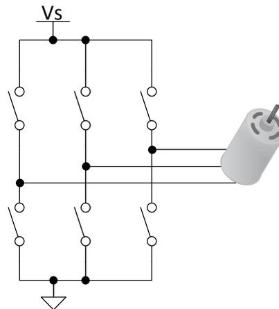
**Figure 1. Simplified Block Diagram of a Three-Phase Motor**
