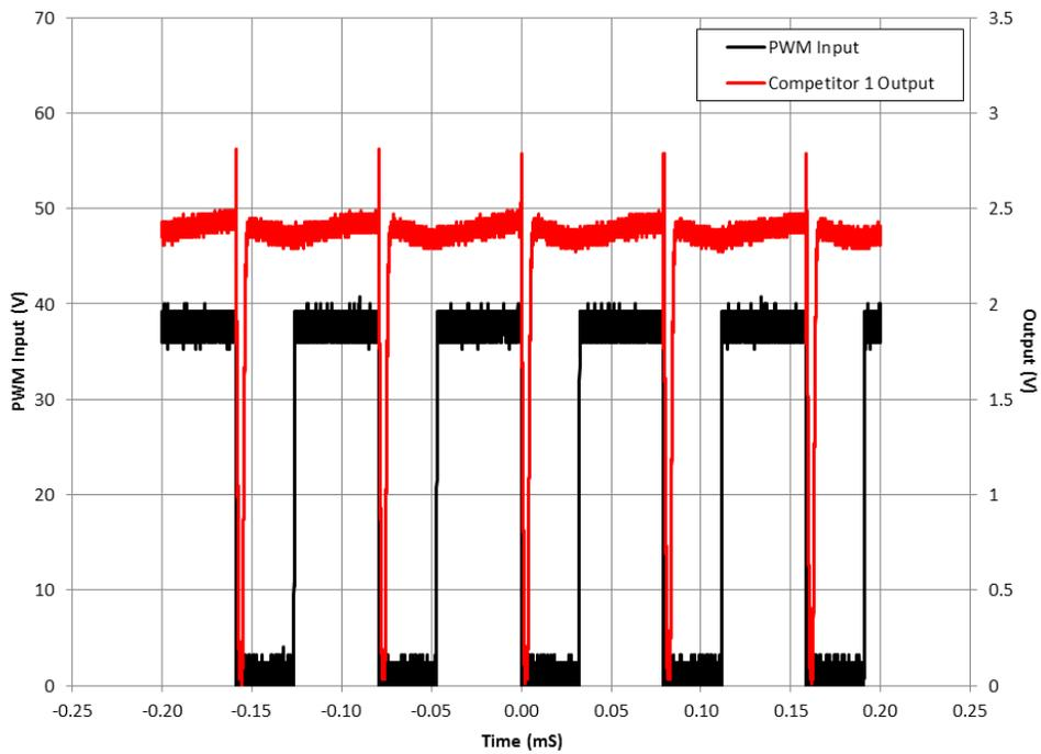
Figure 9. Competitor 1 Output vs PWM Input
