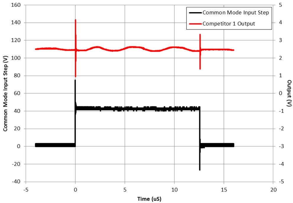
**Figure 6. Competitor 1 Output vs 40-V Common-Mode Step Input**
