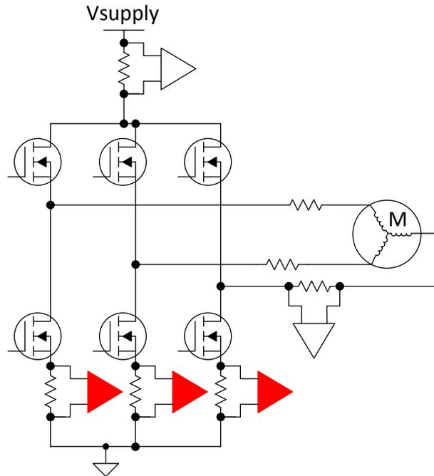
Figure 2. Low Side Implementation of Current Sensing Amplifiers
