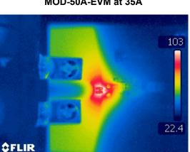
Figure 3-9. Worst-Case Thermal Results With Forced Air Cooling: AMC-MOD-50A-EVM at 50A
