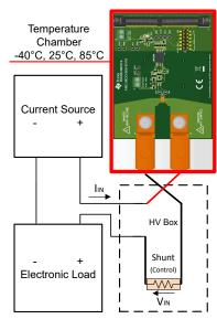
Figure 3-1. Positive Current Equipment Setup
