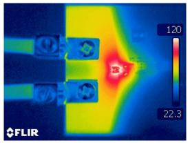
Figure 3-8. Worst-Case Thermal Results: AMC-MOD-50A-EVM at 50A
