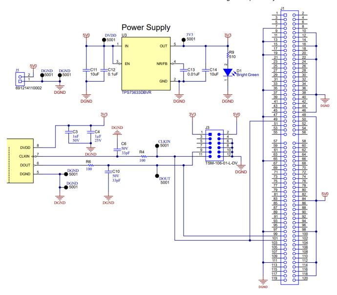
Figure 2-3. AMC-MOD-50A-EVM Digital Interface
