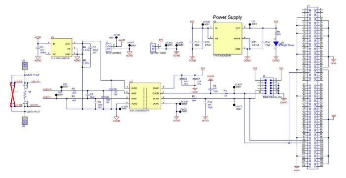
Figure 4-1. AMC-MOD-50A-EVM Schematic
