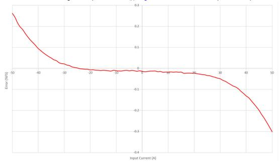
Figure 3-4. AMC-MOD-50A-EVM Total Error %FS Results
