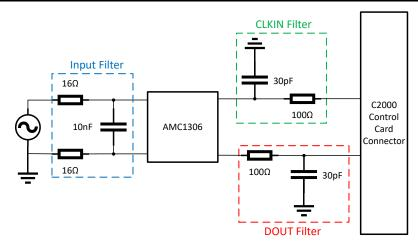
Figure 3-5. AMC-MOD-50A-EVM Filter Diagram
