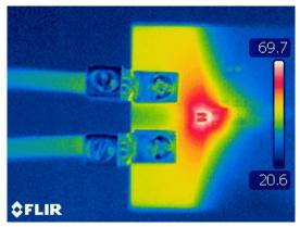
Figure 3-7. Typical Thermal Results: AMC-MOD-50A-EVM at 35A
