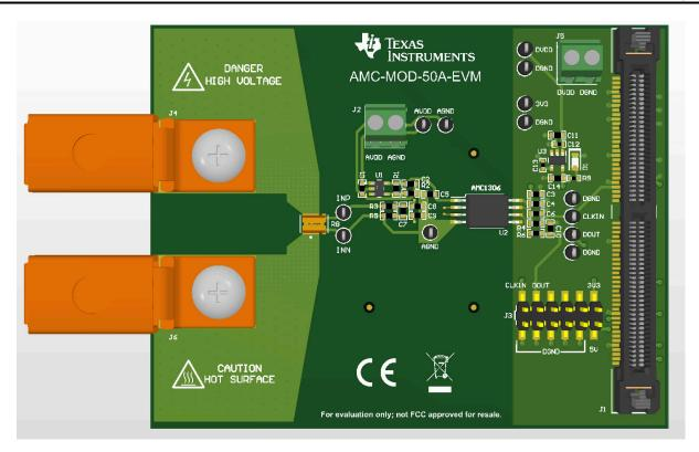
Figure 4-2. AMC-MOD-50A-EVM Top PCB Drawing
