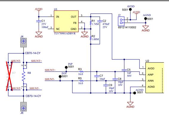
Figure 2-2. AMC-MOD-50A-EVM Analog Input
