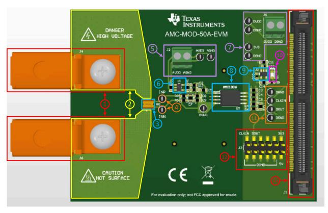
Figure 2-1. AMC-MOD-50A-EVM Hardware Labels
