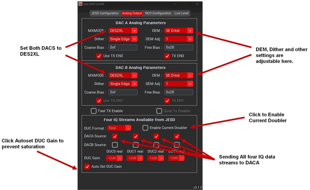
Figure 2-18. DAC39RF12EVM GUI Configuration Steps, Step 4
