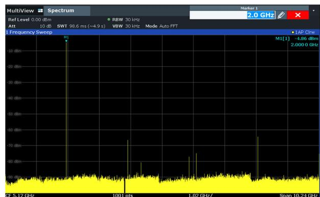
DACB Generating a 2GHz tone in DDS mode. Note the reduced 2<sup>nd</sup> Nyquist image due to DES2XL output mode
