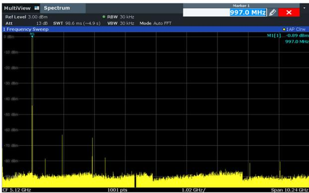
DACA Generating a 1GHz tone in DDS mode. Note the reduced 2<sup>nd</sup> Nyquist image due to DES2XL output mode
