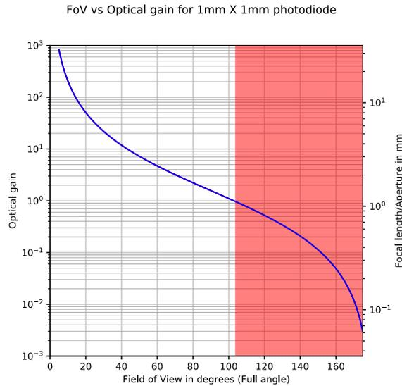
**Figure 24. Field of view vs optical gain**
