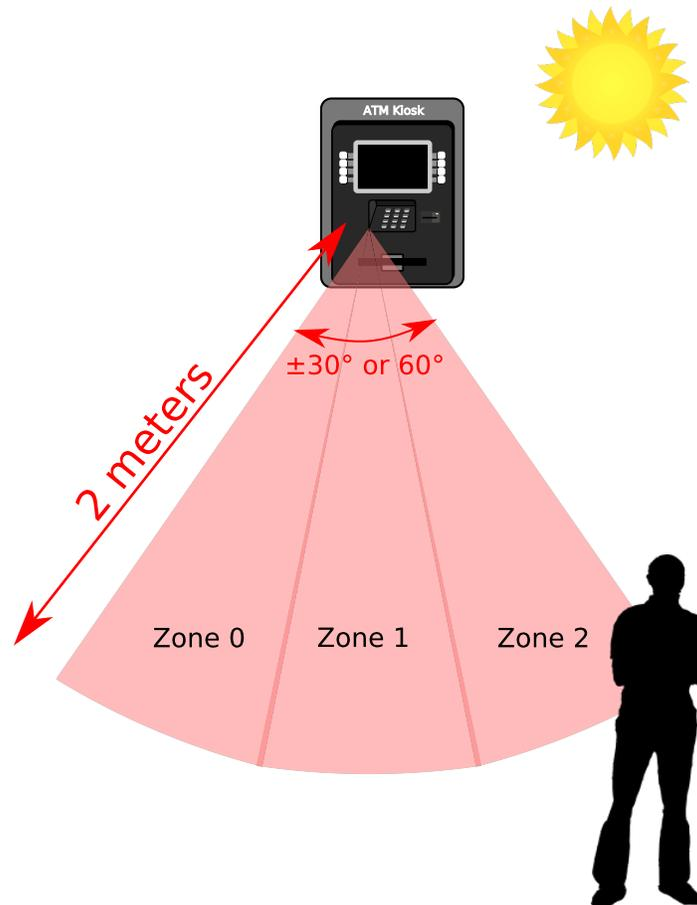
**Figure 5. ATM Kiosk person detection system**
