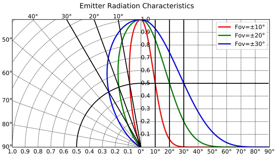
Figure 13. Angular Emissions of LEDs With Various FoVs
