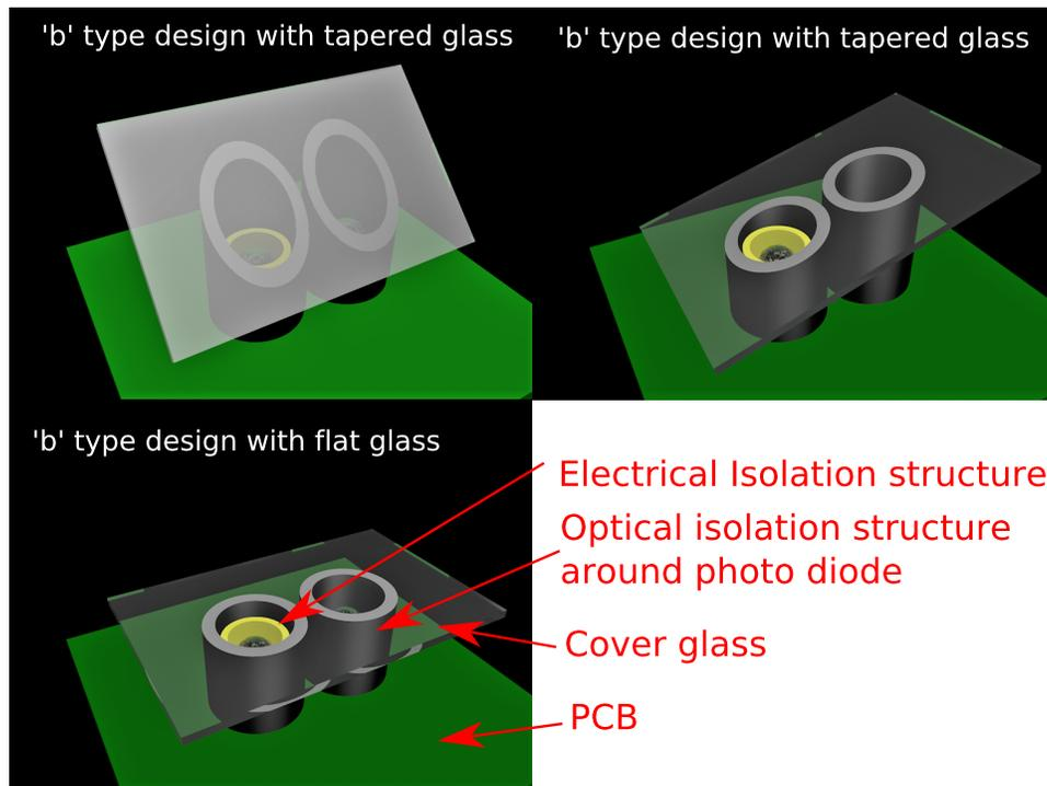
**Figure 19. Dual cavity common glass 3D example**
