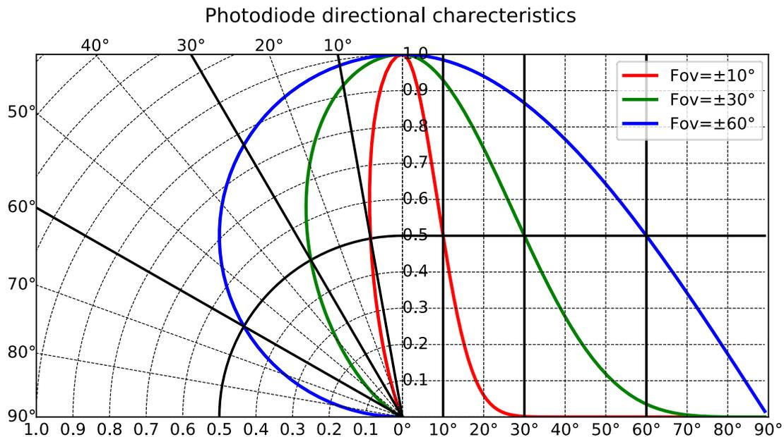
Figure 12. Angular Responses of Photodiodes With Varying FoVs
