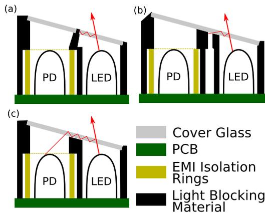
Figure 17. Cover glass design for angled glass
