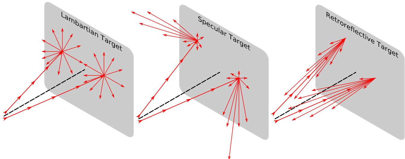
**Figure 8. Type of Targets Based on Reflectance**
