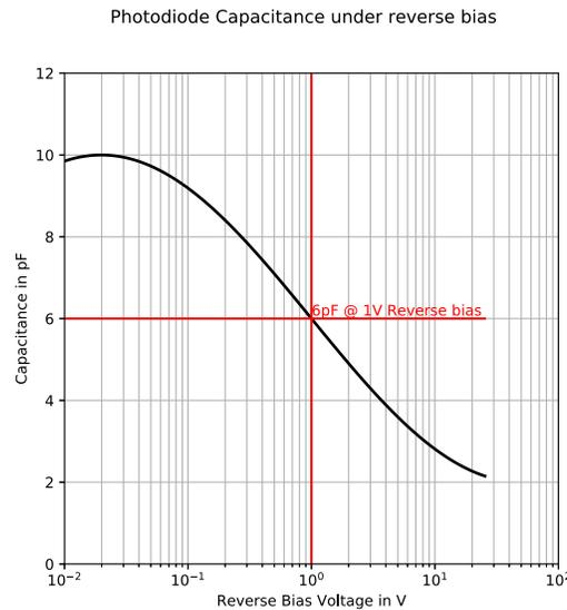
**Figure 11. Reverse Biased Junction Capacitance Curve of Photodiode**
