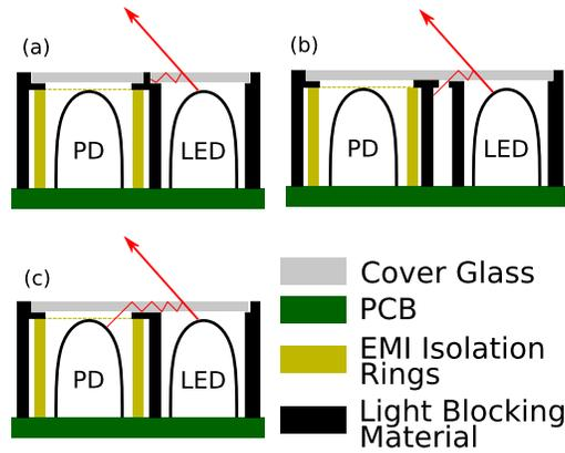
Figure 16. Cover glass design for flat cover glass
