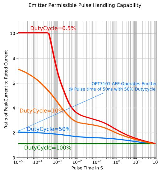
**Figure 14. Duty Cycle Thermal Limit Curve for LED**
