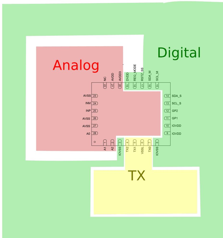
**Figure 28. PCB sections recommended**
