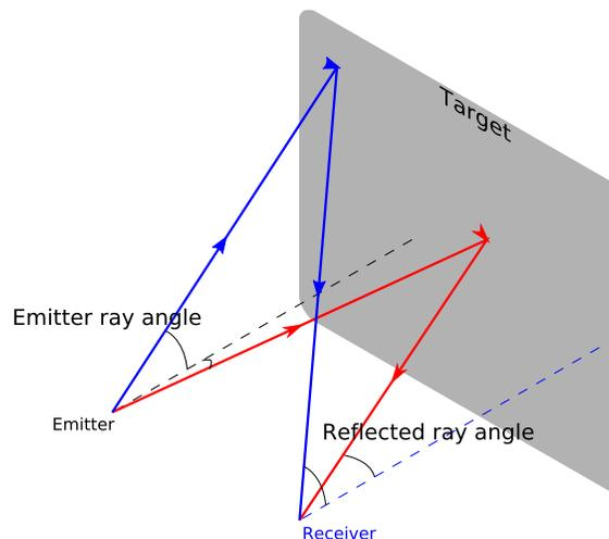
**Figure 15. Ray diagram of transmit and receive light**
