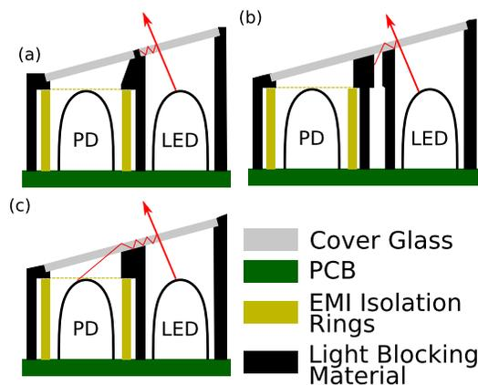
Figure 18. Cover glass design for angled glass
