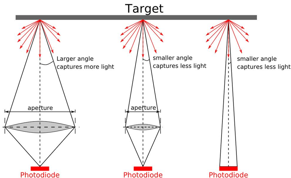
**Figure 20. Receiver Optics with and without Lens**
