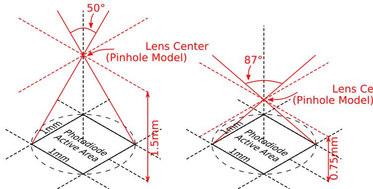
Figure 23. Field of View with pin hole model
