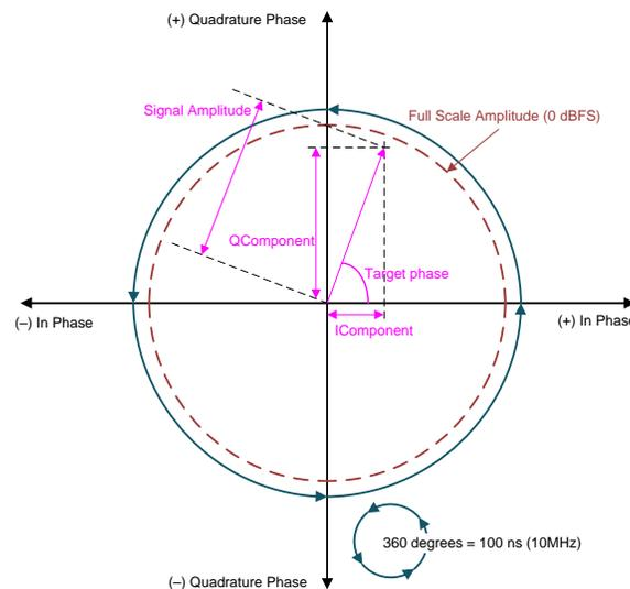
Figure 3. Vector Diagram Representation for ToF Signal
