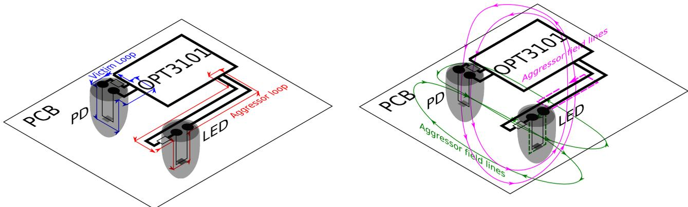
**Figure 27. PCB Layout with magnetic field lines**
