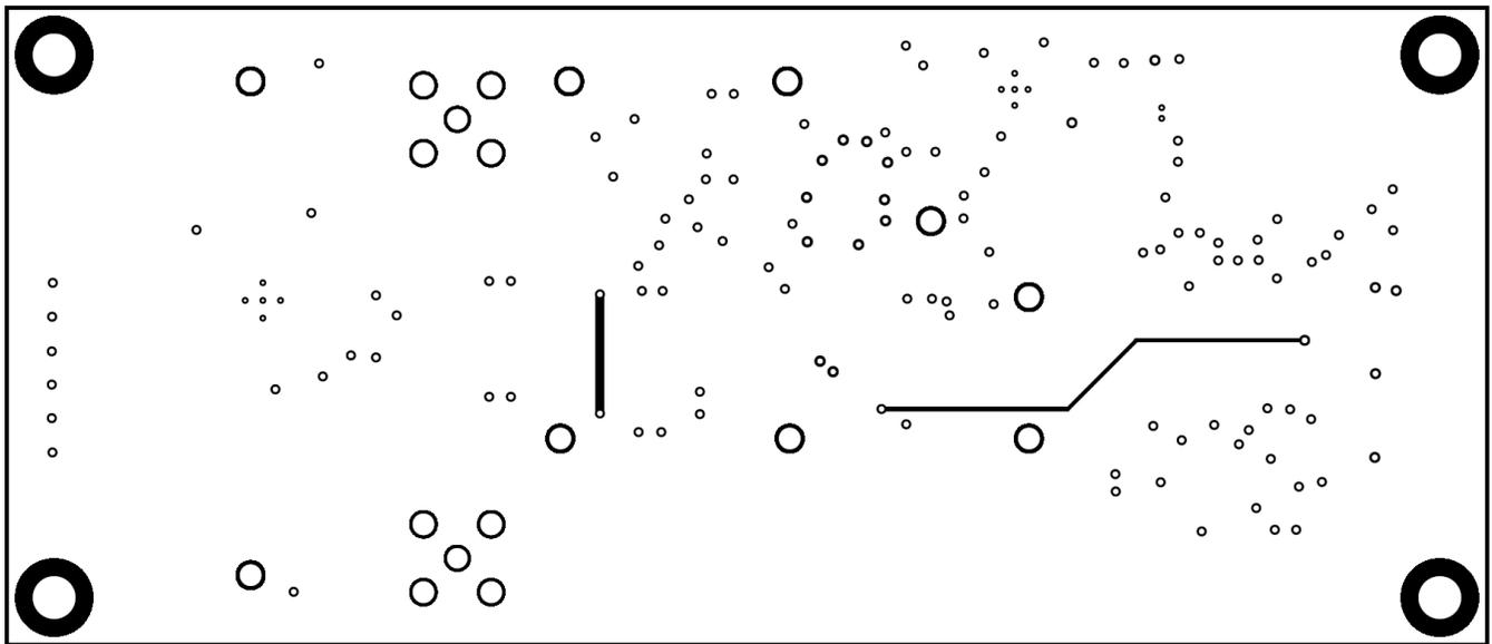
Figure 16. REF6025EVM PCB Layer 4: Bottom Layer
