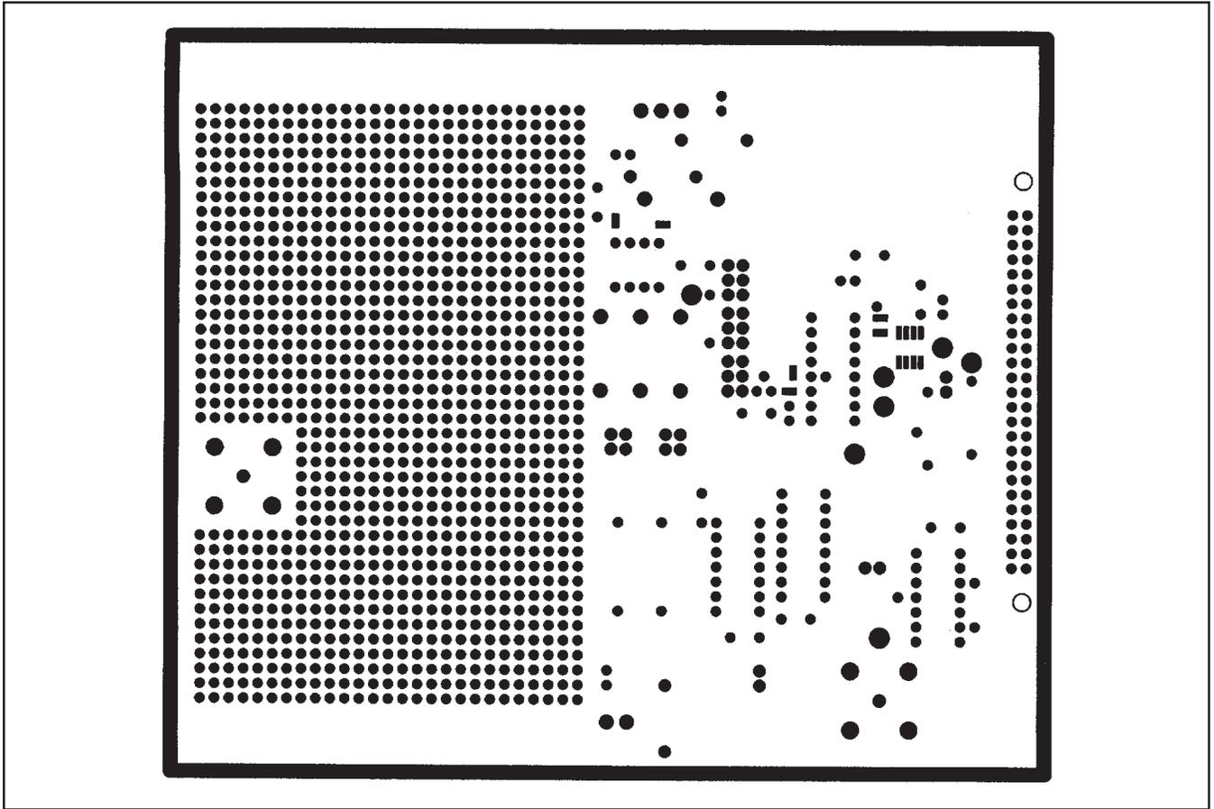
FIGURE 5. Top Soldermask of the DEM-ADS7812/13P Demonstration Board.
