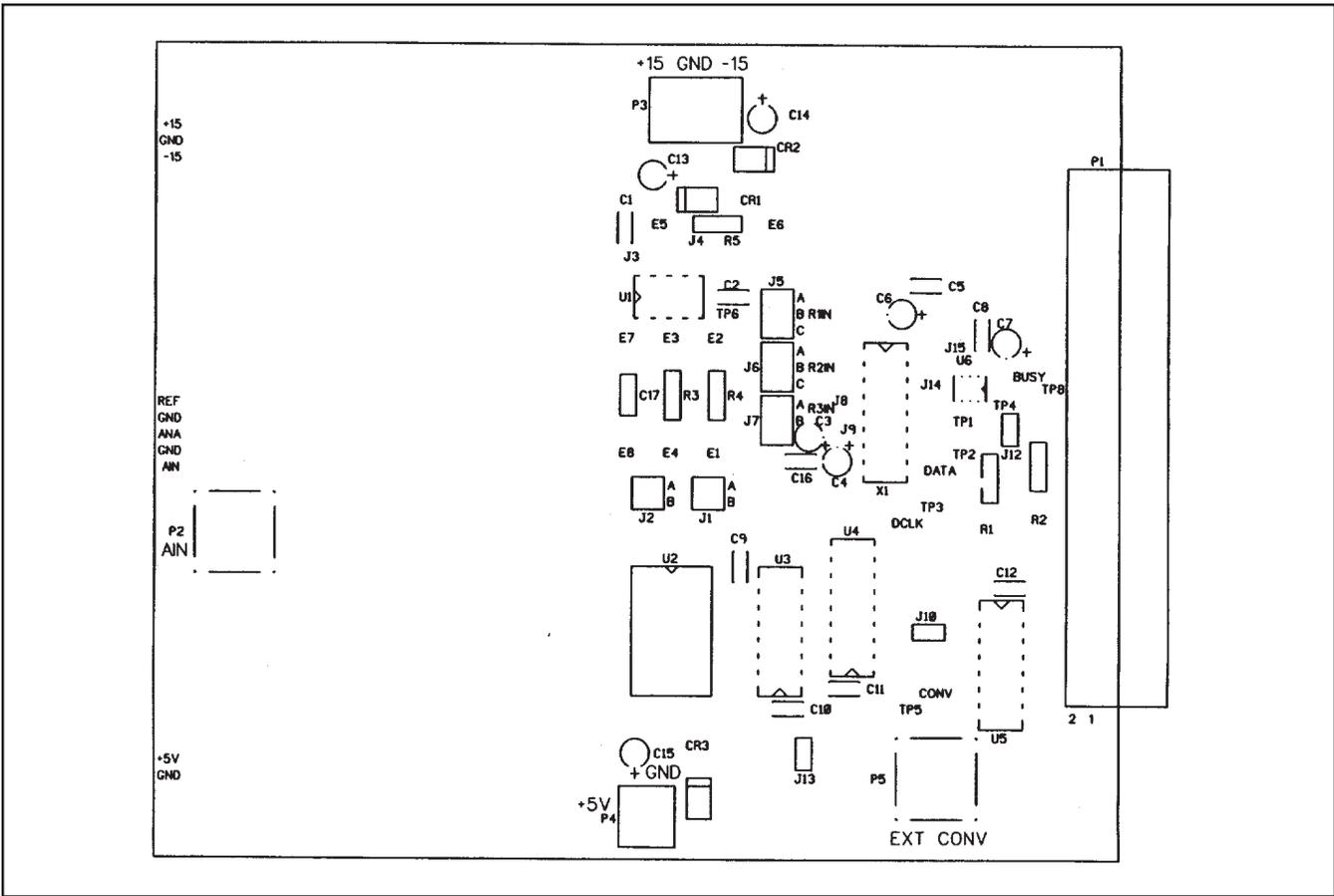
FIGURE 3. Silkscreen of the DEM-ADS7812/13P Demonstration Board.
