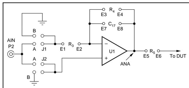
FIGURE 1. The Analog Input Section of the DEM-ADS7812/13P Demonstration Fixture.
