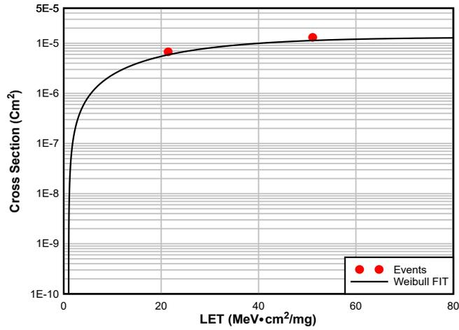
**Figure 8-1. Cross Section Plot for Total Events**
