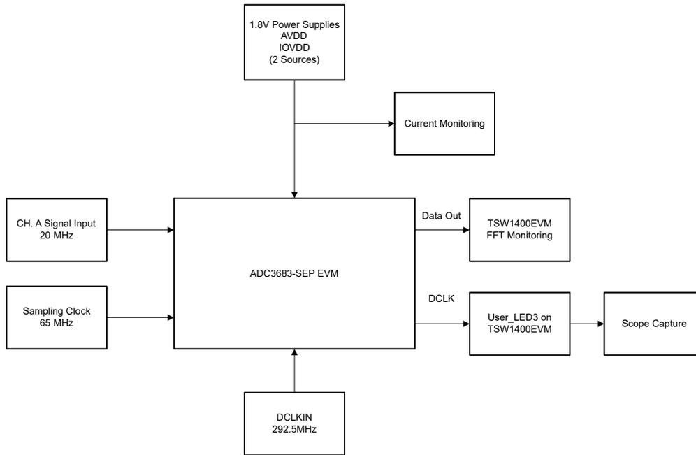
**Figure 5-1. Block Diagram of SEE Test Setup With the ADC3683-SEP**
