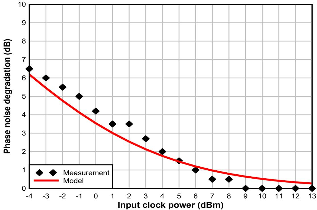
Figure 4-1. Impact of Clock Input Power on Flicker Noise for LMX2615-SP PLL
