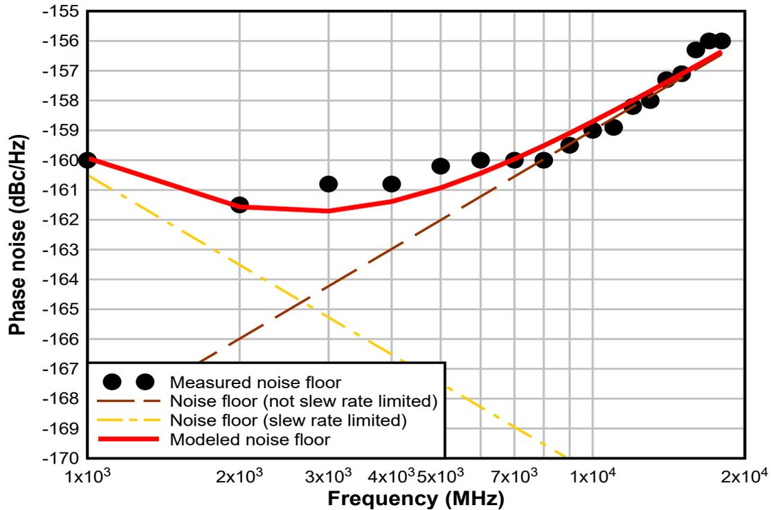
Figure 3-3. LMX1214 Noise Floor Trends vs. Frequency
