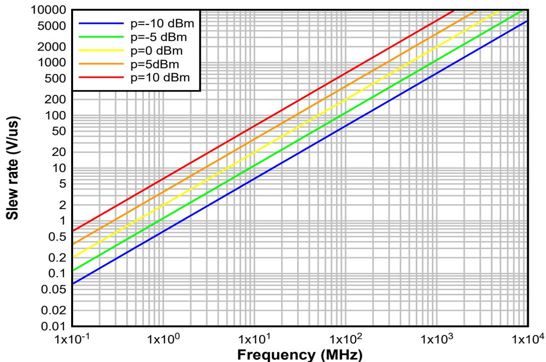
Figure 2-1. Relationship Between Power, Slew Rate, and Frequency for a Sine Wave
