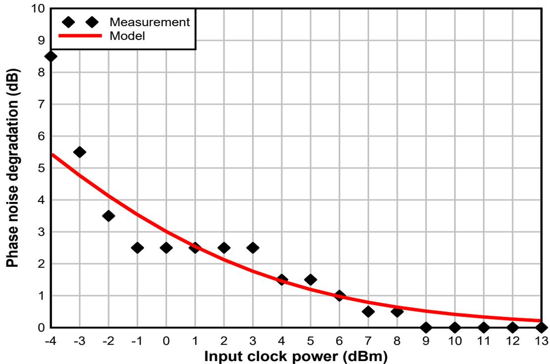
Figure 4-2. Impact of Clock Input Power for PLL Figure of Merit for LMX2615-SP PLL
