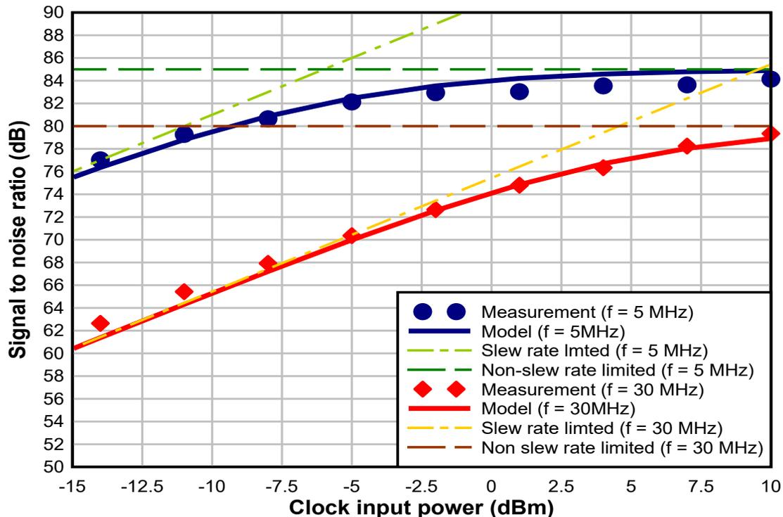
**Figure 5-1. Data Converter SNR vs Input Clock Power for Rohde and Schwarz SMA100B Signal Generator**
