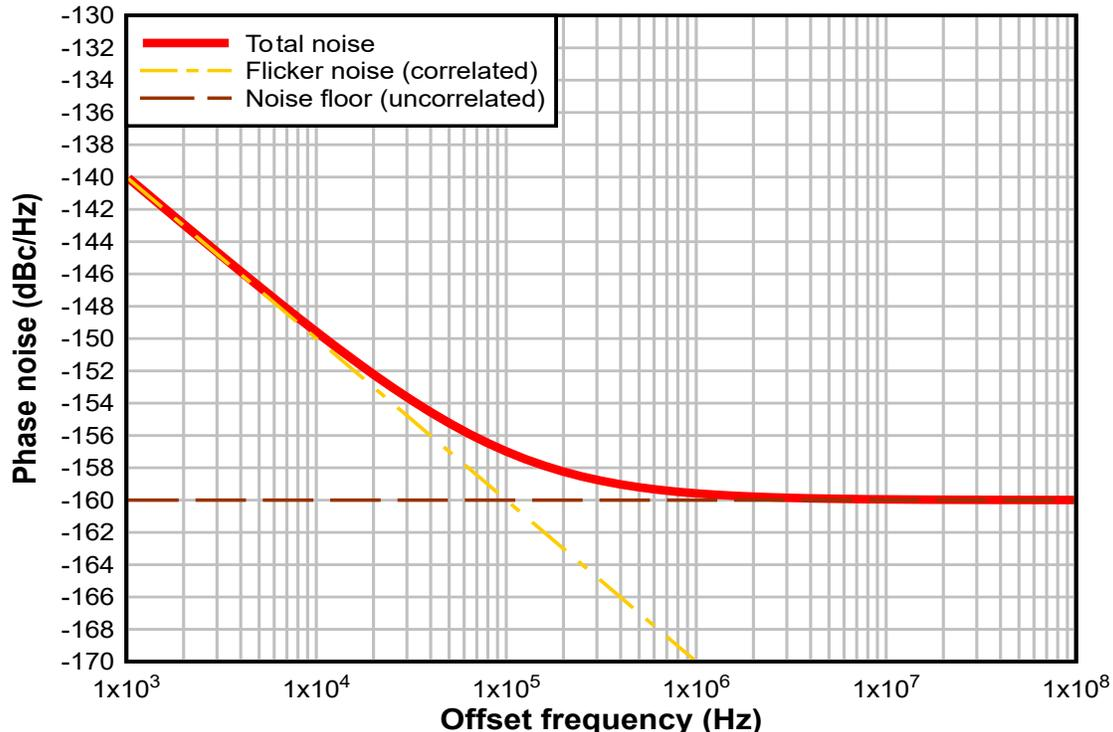
Figure 1-1. Calculation of Total Noise From Flicker Noise and Noise Floor
