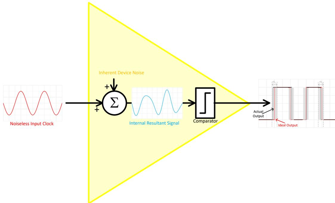
**Figure 3-1. Modeling Impact of Slew Rate on Output Jitter**
