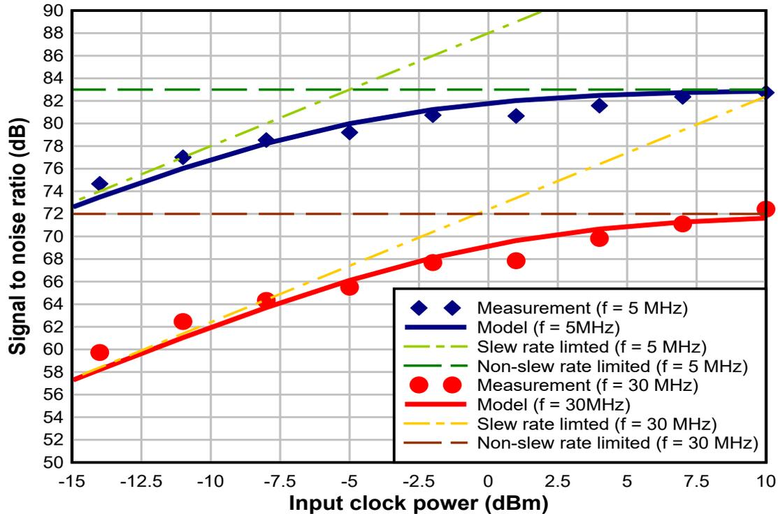
Figure 5-2. Data Converter SNR vs Input Clock Power for Agilent 4438C Signal Generator
