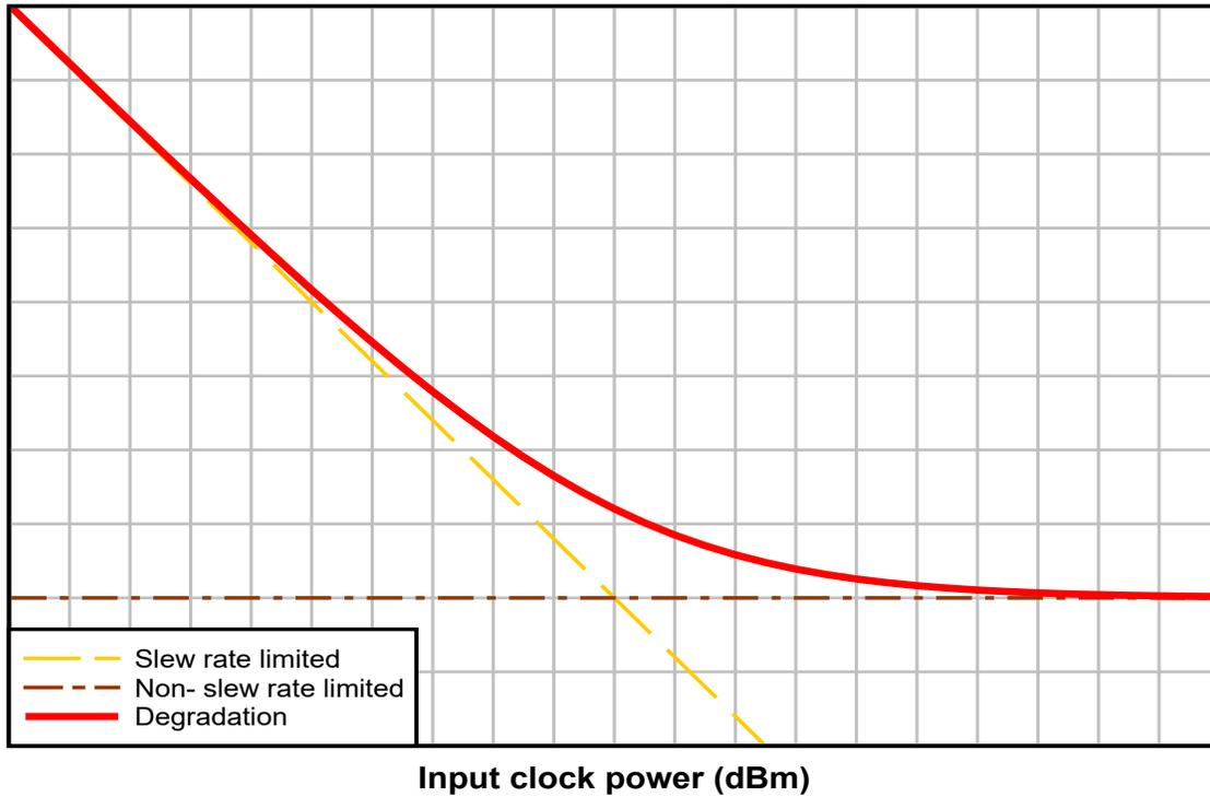
**Figure 3-4. Phase Noise Degradation as a Function of Slew Rate**
