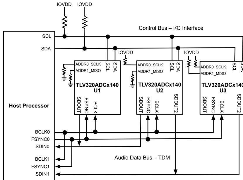
**Figure 3-11. TLV320ADCx140/PCMX140-Q1 Shared Split TDM With Primary and Secondary Bus Connection Diagram**
