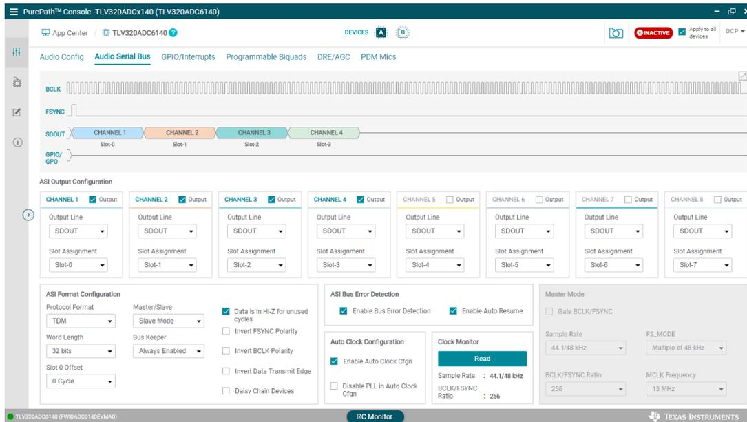
Figure 4-5. PurePath Console Device A Channel to Slot Mapping
