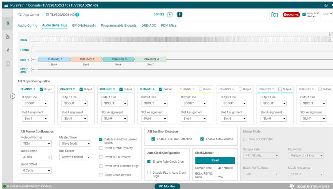
Figure 4-6. PurePath Console Device B Channel to Slot Mapping
