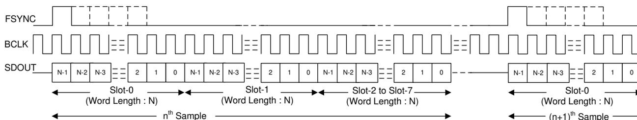
**Figure 3-1. TDM Mode Standard Protocol Timing (TX\_OFFSET = 0)**
