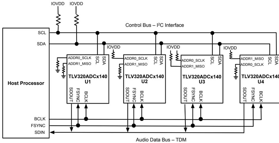
Figure 3-2. TLV320ADCx140/PCMX140-Q1 Shared TDM Connection Diagram
