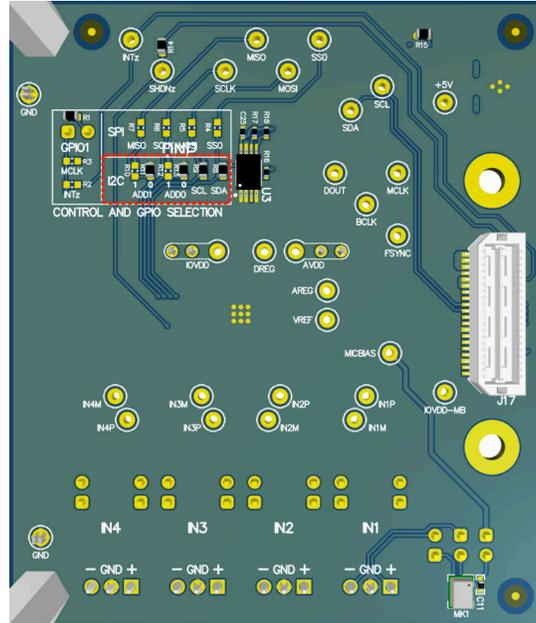
**Figure 4-2. I<sup>2</sup>C Address Configuration for the TLV320ADx140 EVM**
